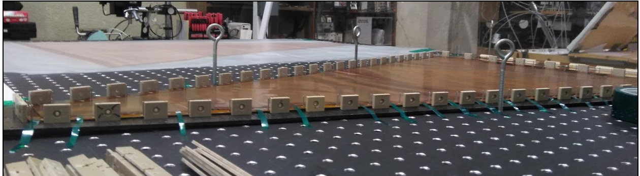
Figure 3: Tape keeping tension on the ROB (second rebuild)
