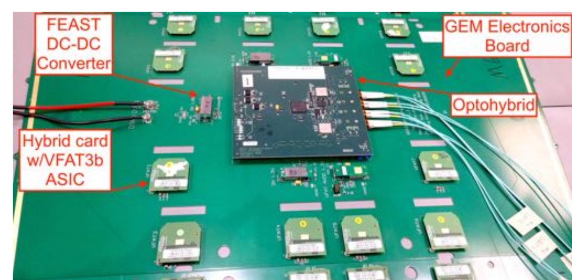
Figure 4: A GE2/1-M6 GEM electronics board with prototype frontend electronics.
