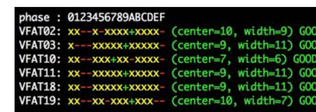
Figure 9: Phase scan results for the second OH on the wide ME0 GEB.
