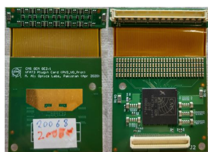
Figure 6: The front (left) and back (right) of the plugin card with VFAT3b ASIC.
