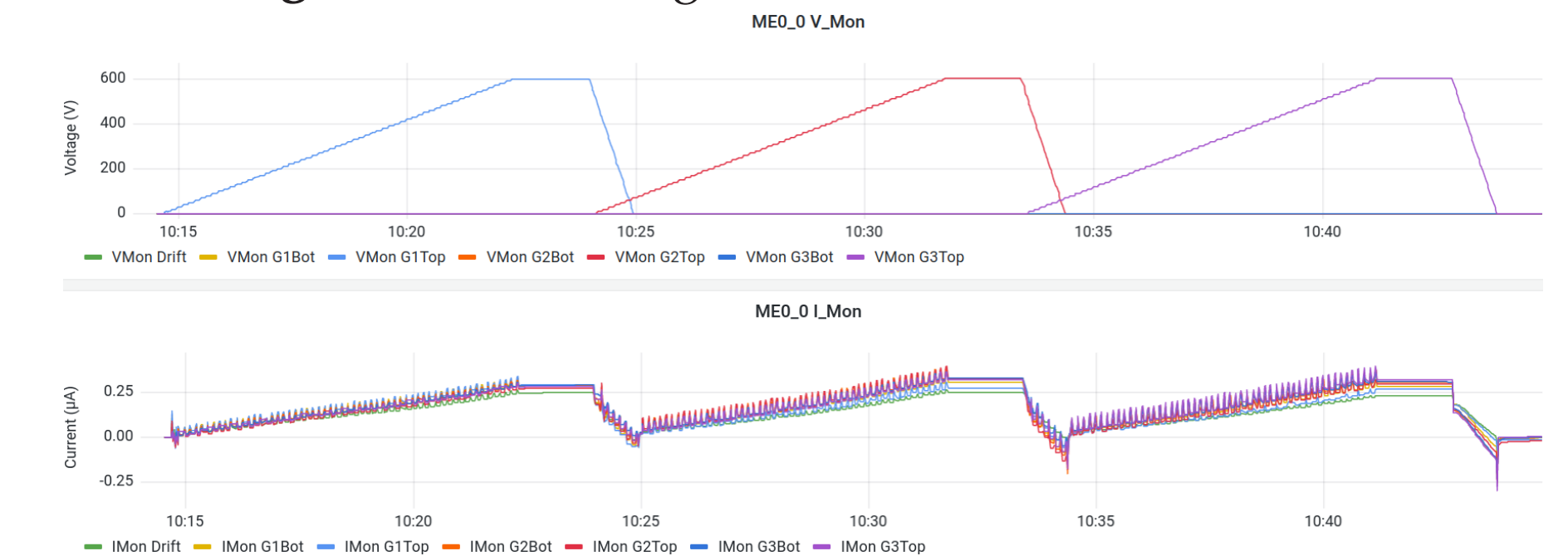
Figure 6: Current leaks in ME0 HV filter during Stress Test at FIT.
