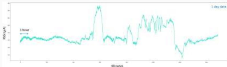
RSSI monitoring over 24 hours; range of 272–286  $\mu\text{A}$  [3].
