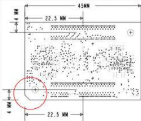
Corner of PCB will be cut to avoid connecting to GEB in the incorrect orientation [5].
