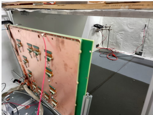
The M5 module inside the X-ray box for the effective gain measurement
