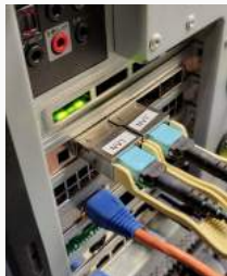
Optical transceivers plugged into the CVP13
