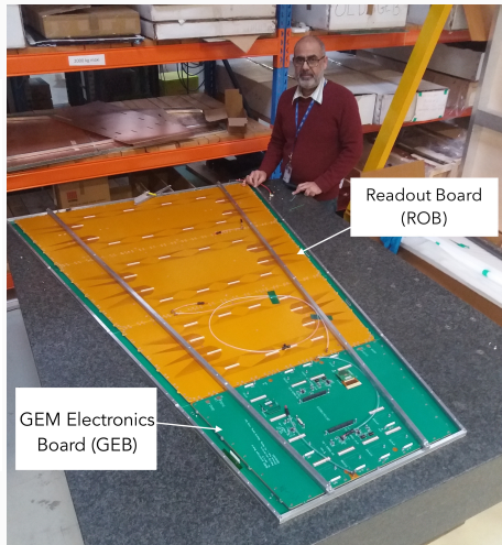
First fully assembled GE2/1 chamber [2].
