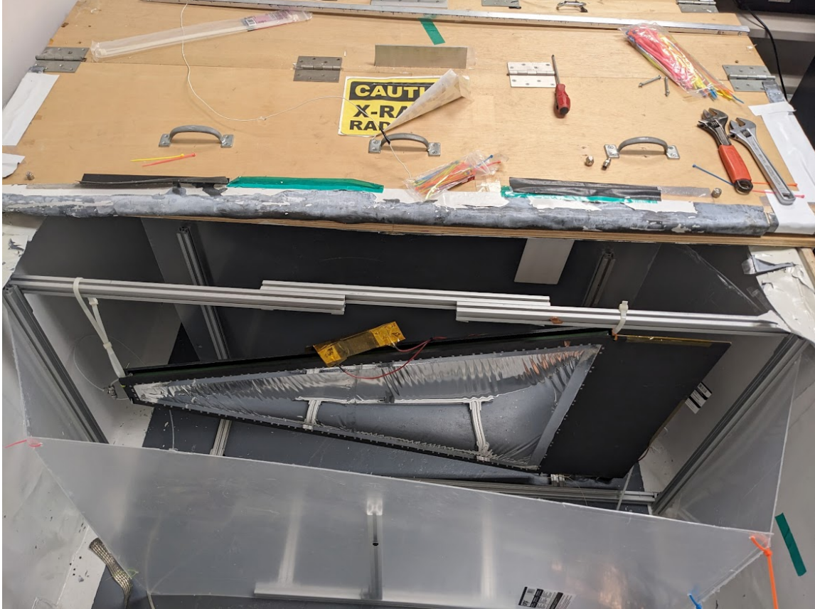
Figure 1: LMG detector inside the X-ray box. The LMG is surrounded by acrylic shielding to protect from high voltages. During operation, an additional sheet of acrylic rested over the LMG so that it is completely enclosed. Additionally, it can be seen that the GEM foil is properly inflated.
