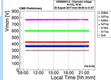
Similar results have been observed for the LV system **Right:** stability within 10-<sup>3</sup>, observed in a 12 hours period during collisions with the multichannel HV system
