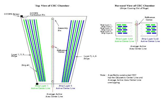
• The Simulated CSC Chamber Geometry and Local Coordinate System in the Idealized COCOA Model. The 'Average Active Center' of the CSC chambers is taken as the Reference Center for COCOA EMU simulations.
