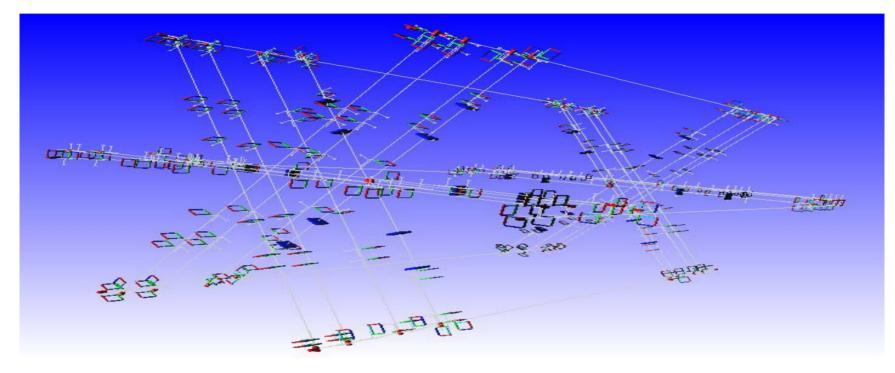
The Simulated EMU Alignment System. This is a COCOA generated VRML representation of the simulated geometry used for the idealized simulations of the EMU Alignment System.
