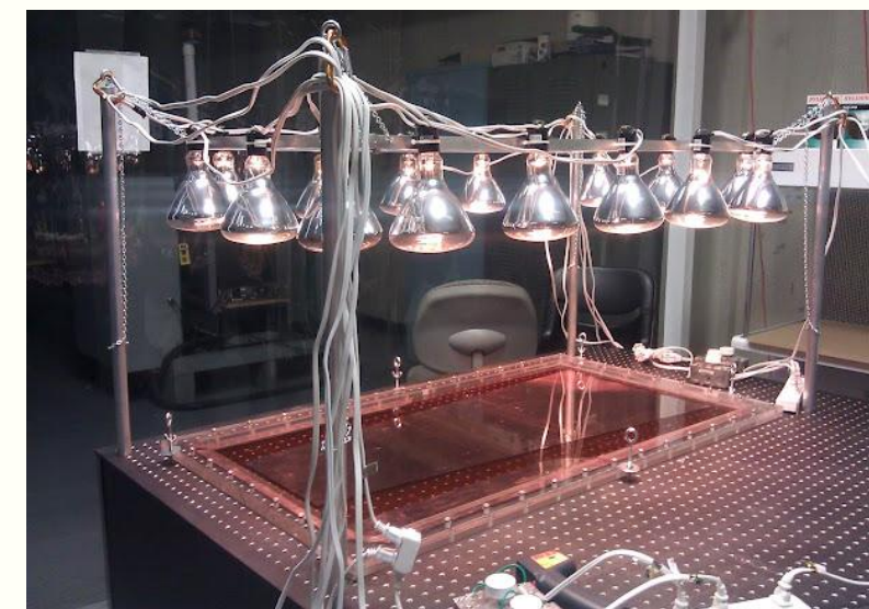
Figure 3: The modified infrared stretching array
