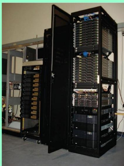
**Figure 1:** The Florida Tech Cluster is encased within one 50U rack.
