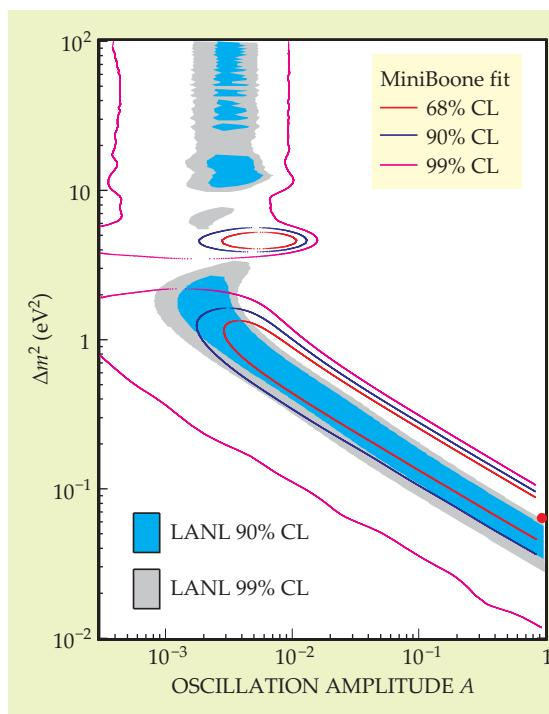
**Figure 2.** Neutrino-oscillation parameters favored by the MiniBooNE and Los Alamos antineutrino-beam experiments are indicated by confidence-level contours in the parameter space of the oscillation amplitude  $A$  and the mass-squared difference  $\Delta m^2$  between the two participating neutrino states. The best MiniBooNE fit (red dot near maximum  $A$ ) is ruled out by null results from reactor experiments that exclude  $A$  bigger than 0.1. (Adapted from ref. 1.)
