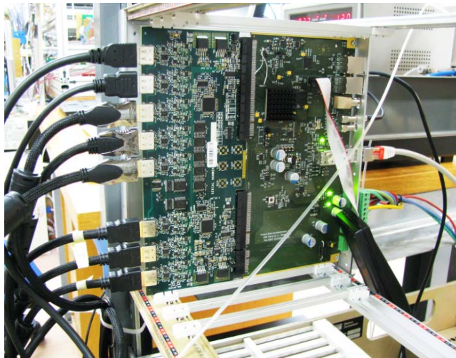
Fig. 13. Photo of powered and fully connected SRS ADC adapter card (left) and FEC card (right) in a 6U chassis.
