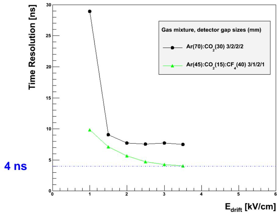
**Using optimized HV divider for standard triple-GEM**
