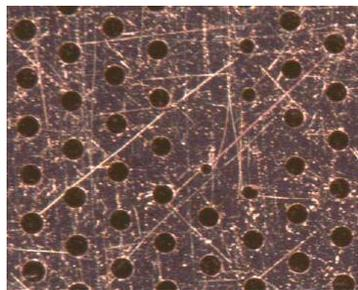
2 defects max,  $< 1 \text{ mm}^2$
