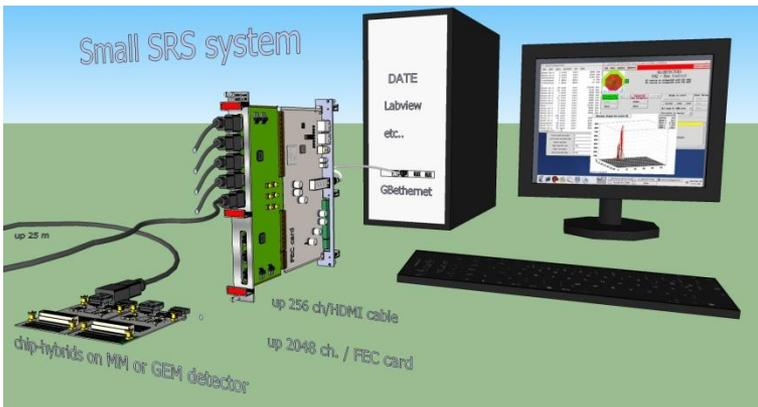
Successful data taking with **analog APV chip** and **Scalable Readout System** in addition to TURBO/VFAT2 DAQ system; allows cog centroid calculation for hit position using **pulse heights**
