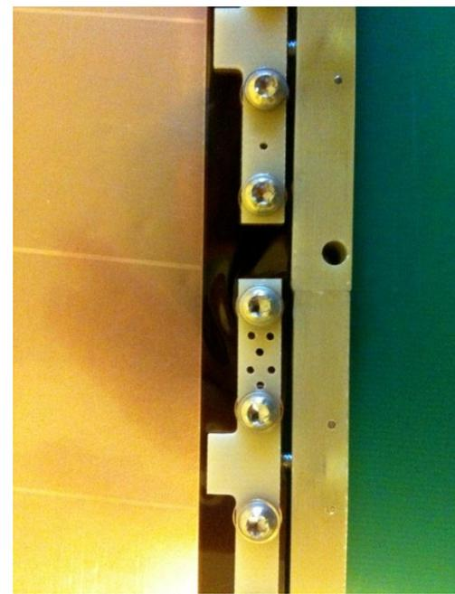
**Allows re-opening of assembled detector for repairs if needed.**
