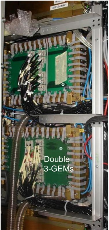
12 Double Triple-GEMs in front of calorimeter; total area 0.6 m<sup>2</sup>
