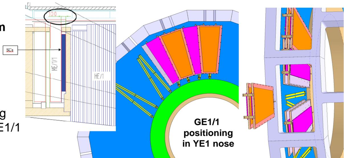
Current GE1/1 production design w/ FE electronics & cooling
