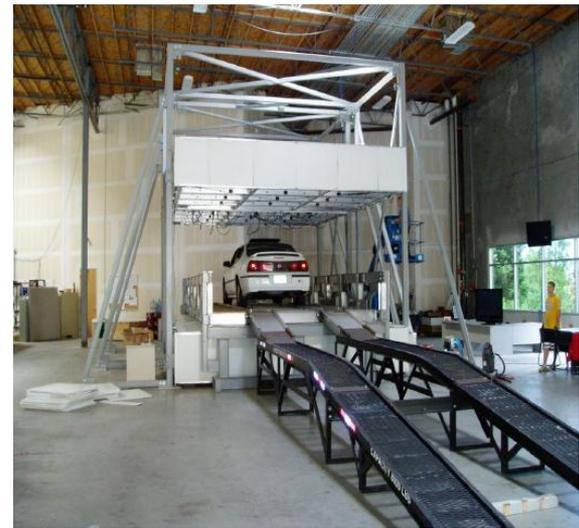
**Decision Sciences prototype using drift tubes large enough to scan a vehicle.**
