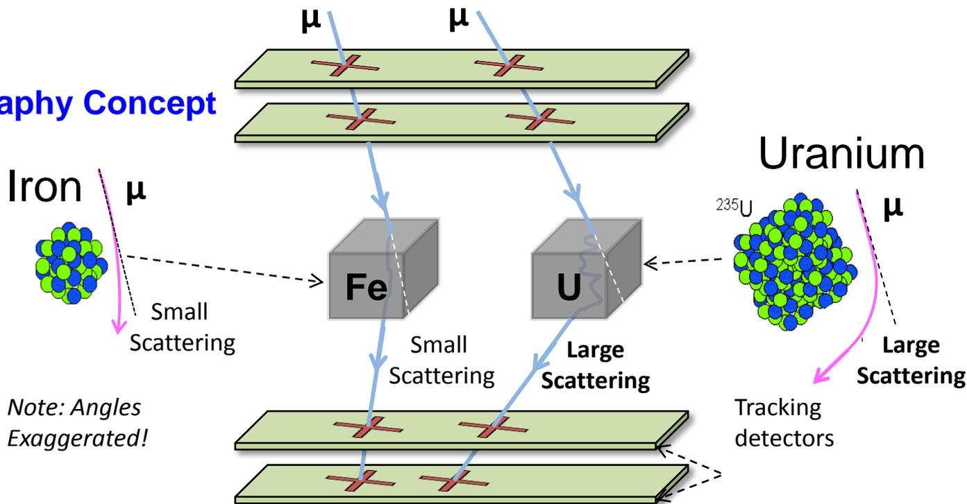
Multiple Coulomb scattering to 1<sup>st</sup> order produces Gaussian distribution of scattering angles  $\theta$  with width  $\sigma = \Theta_0$ :
