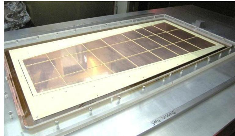
**Single mask GEM foil with spacer frame at CERN (active area: 990 mm long & 220-455 mm wide)**
