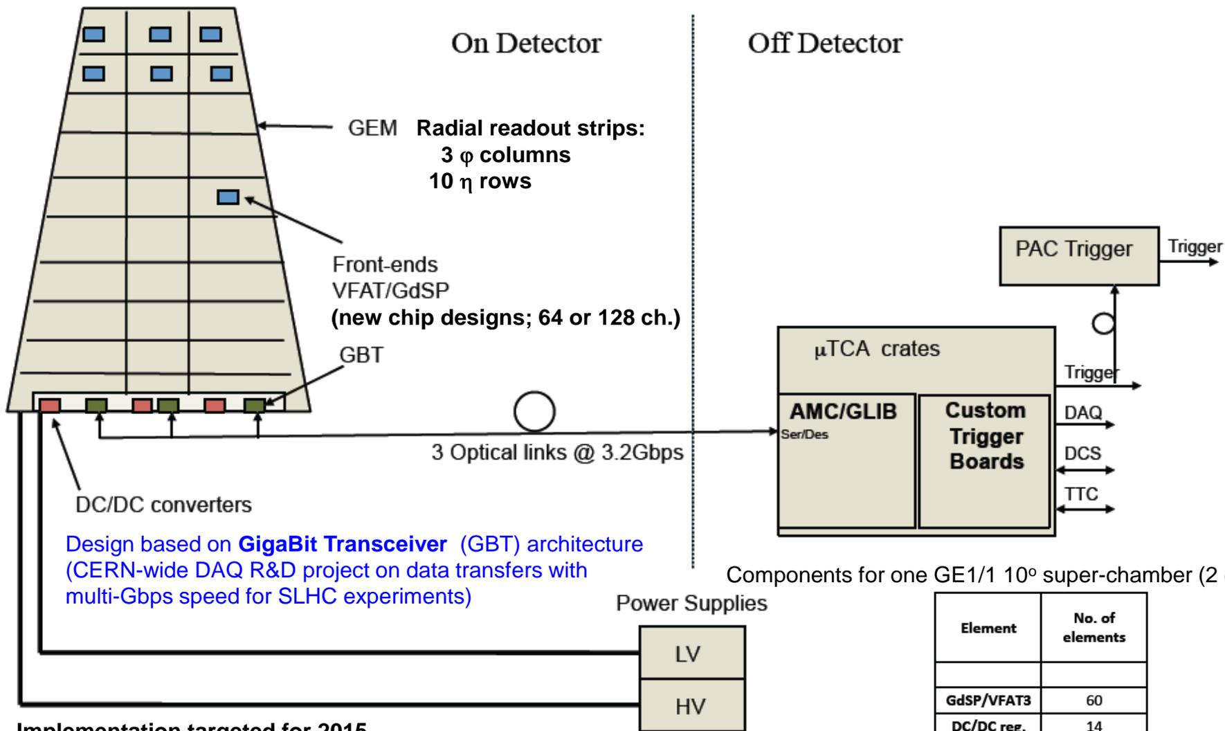
Design based on **GigaBit Transceiver (GBT)** architecture (CERN-wide DAQ R&D project on data transfers with multi-Gbps speed for SLHC experiments)
