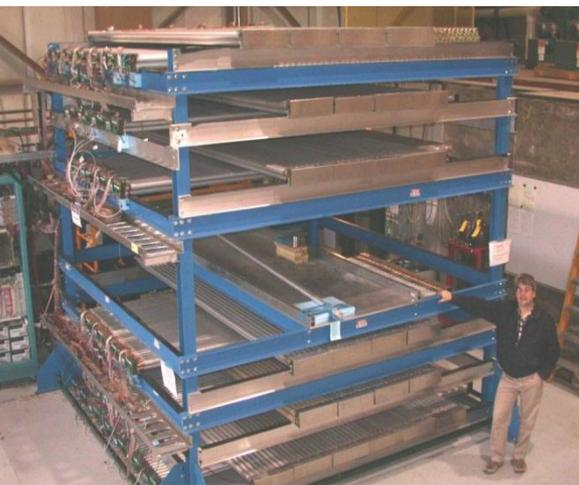
**Original idea from Los Alamos (2003): Muon Tomography with Drift Tubes**
