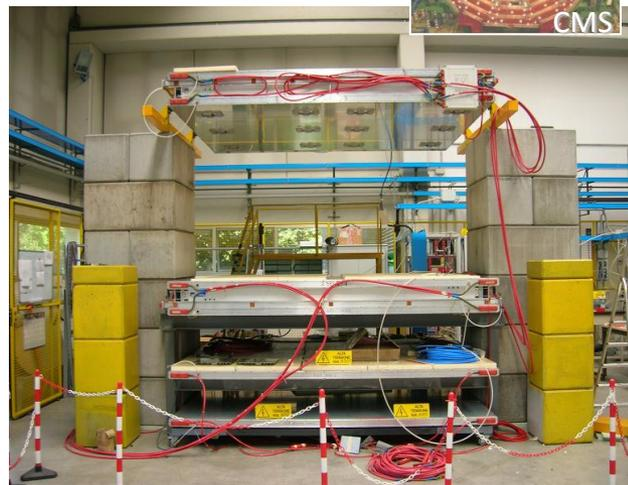
**INFN : Muon Tomography with spare CMS Muon Barrel Chambers (Drift Tubes)**
