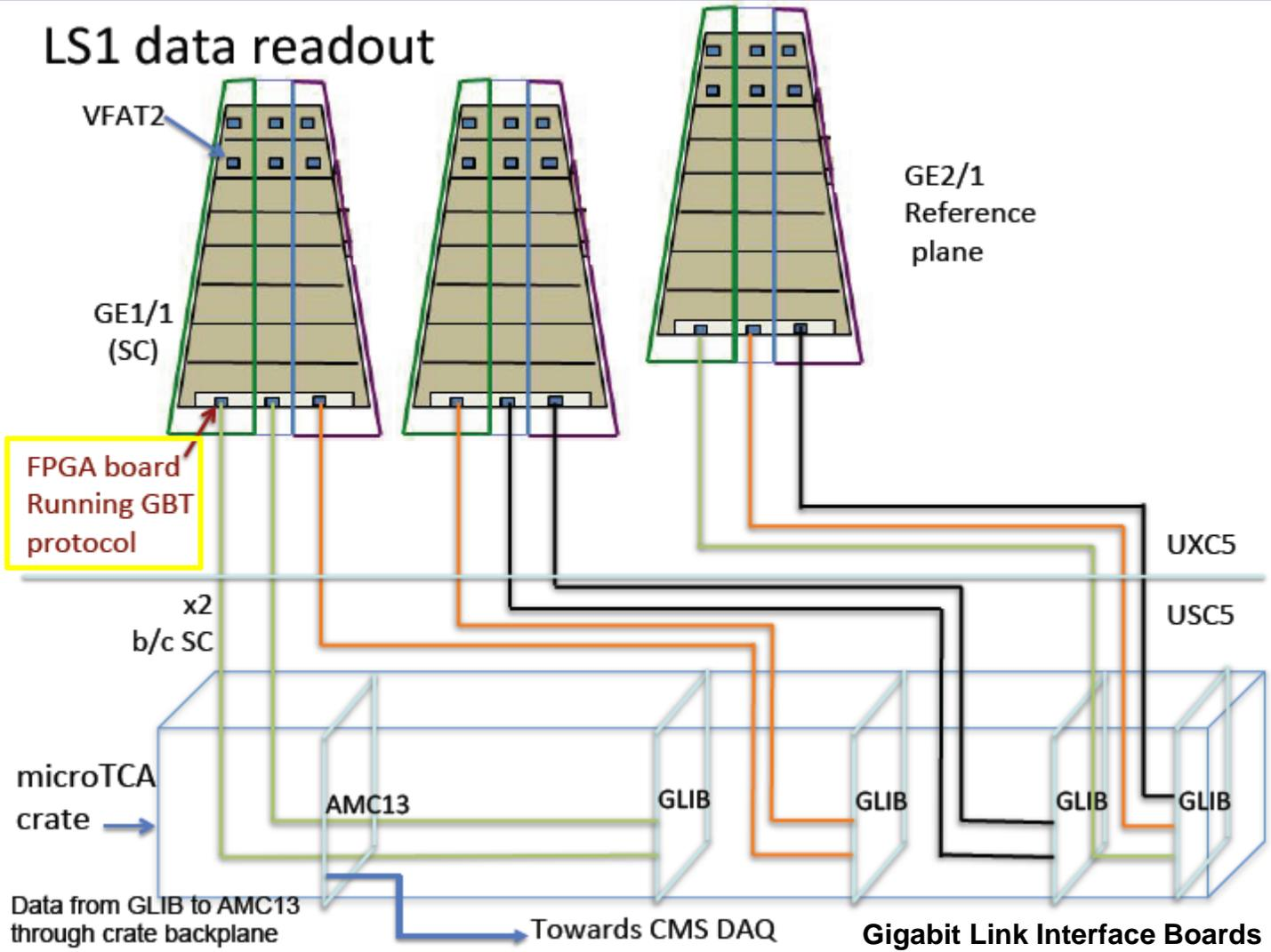
**FPGA also with link to new CSC Trigger Mother Board**
