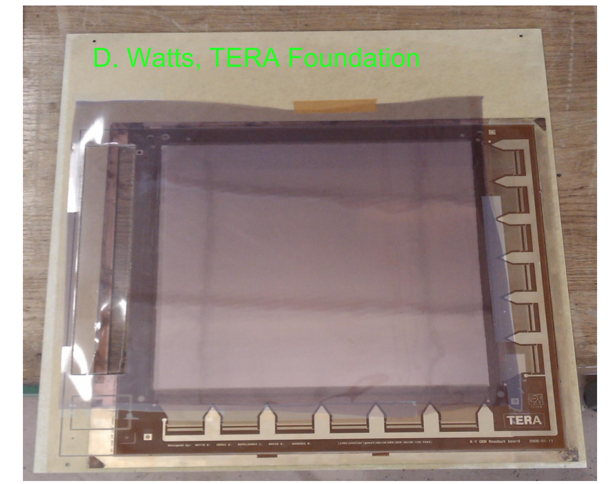
XY readout foil mounted on a honeycomb board
