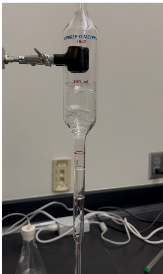
Figure 9: Example of flow rate measurements being performed with a Bubble-O-Meter. The section with a volume of 10 mL can be seen between the two red rings. Currently in the picture, two bubble membranes can be seen flowing upward through this section. Above the highest red ring the 100 mL section starts, and many bubbles can be seen in this section.
