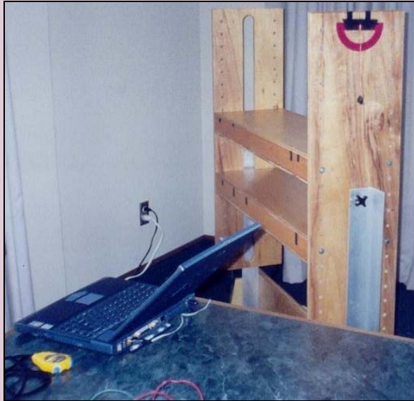
Rotation Mount and Setup for Flux Measurement
