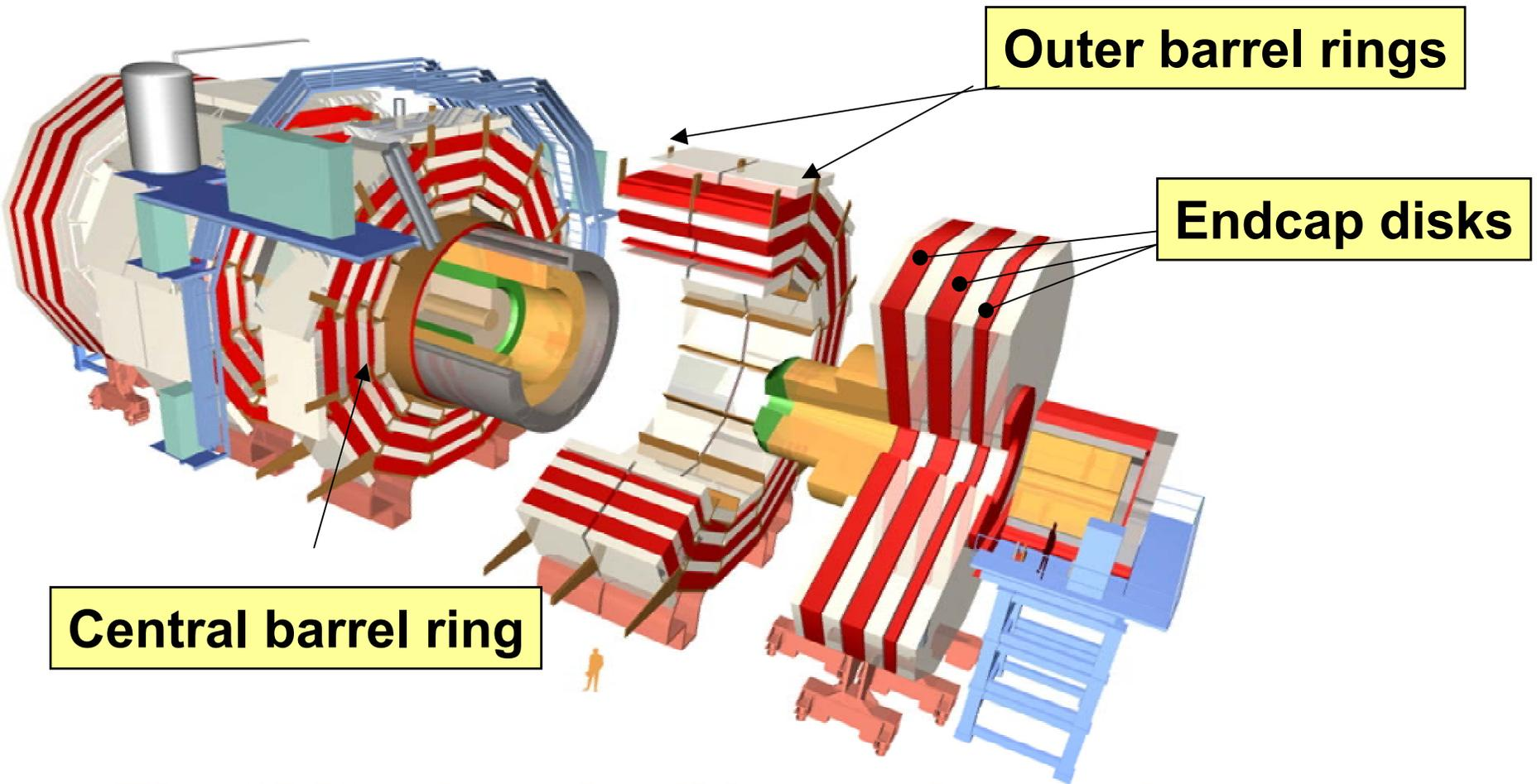
**The CMS solenoid will be 13m long with an inner diameter of 6m – the largest superconducting solenoid ever made!**
