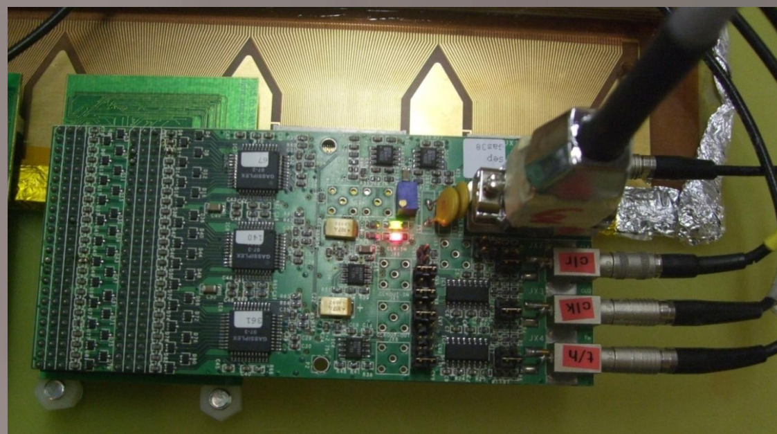
Fig. 7. Gassiplex front-end fully connected and operational.
