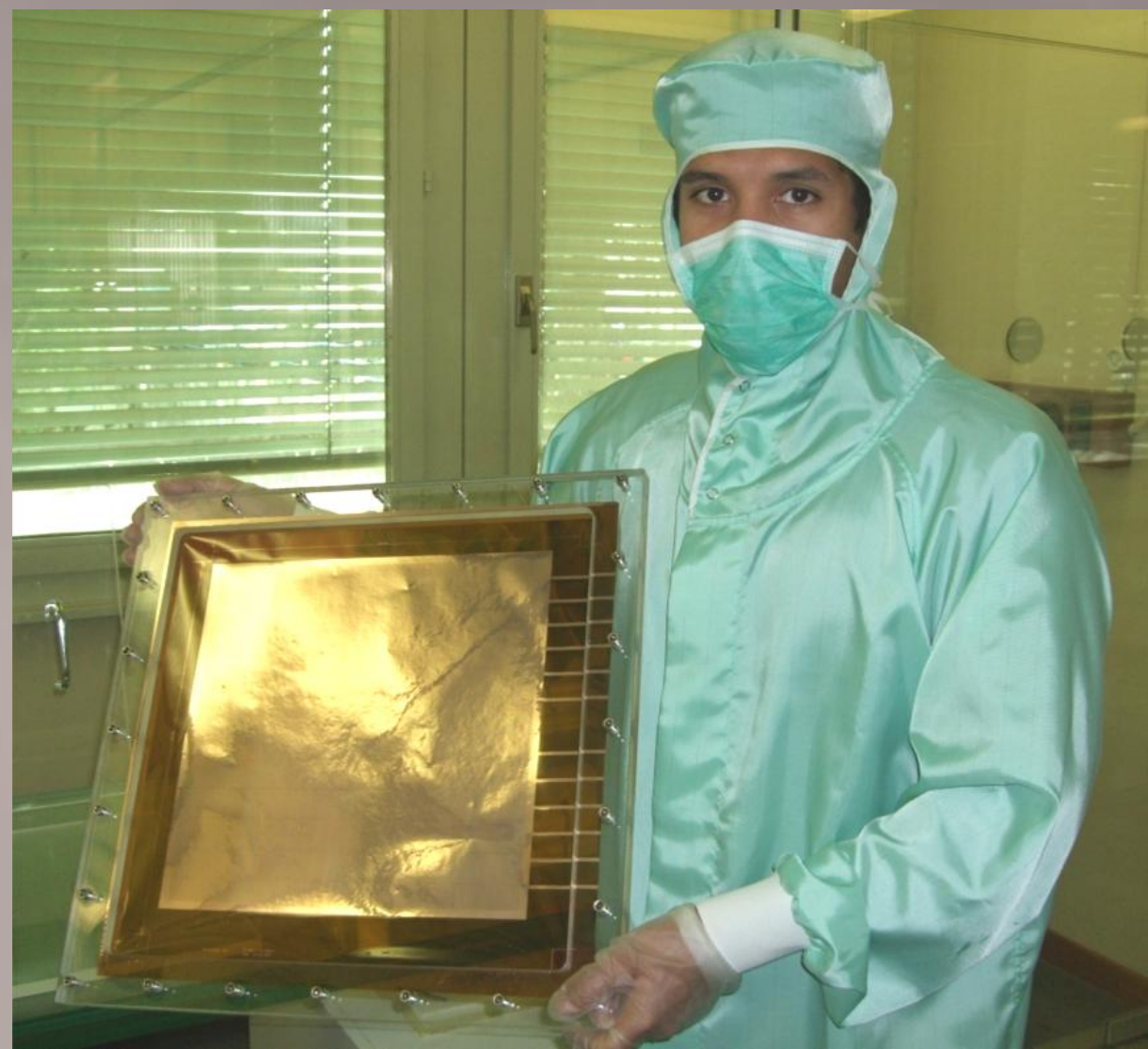
Fig. 4. Foil in stretching device ready to go into oven.
