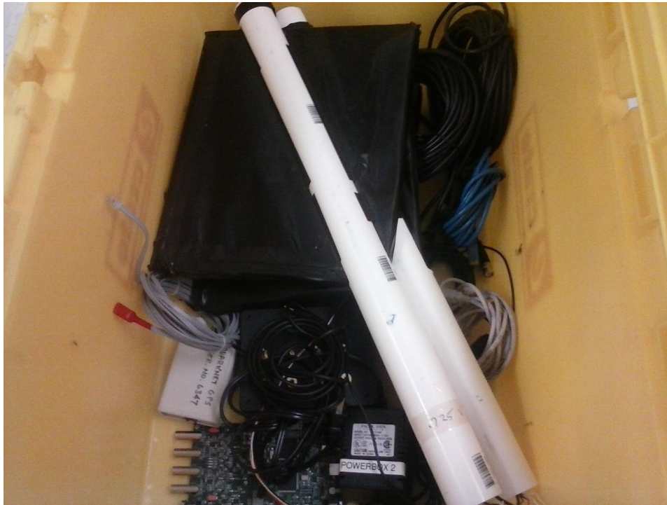
Image 3: Detector paddles with Scintillators and Photomultiplier tubes
