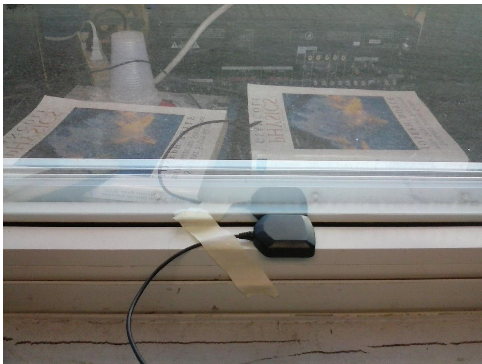
Image 6: GPS Receiver placed at window sill to receive signal from satellites
