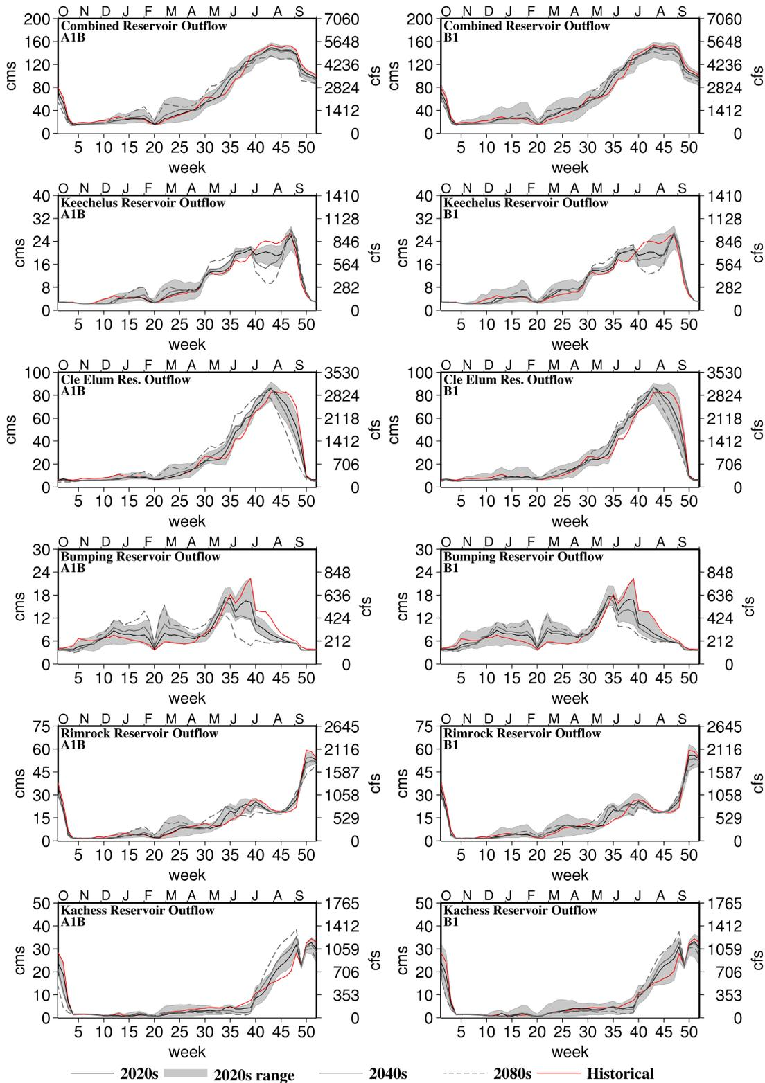
**Figure 8.** Reservoir outflow. Projected reservoir outflow for the combined system (top panel) and for each of the five major reservoirs (lower five panels) for historical, 2020s, 2040s, and 2080s conditions.
