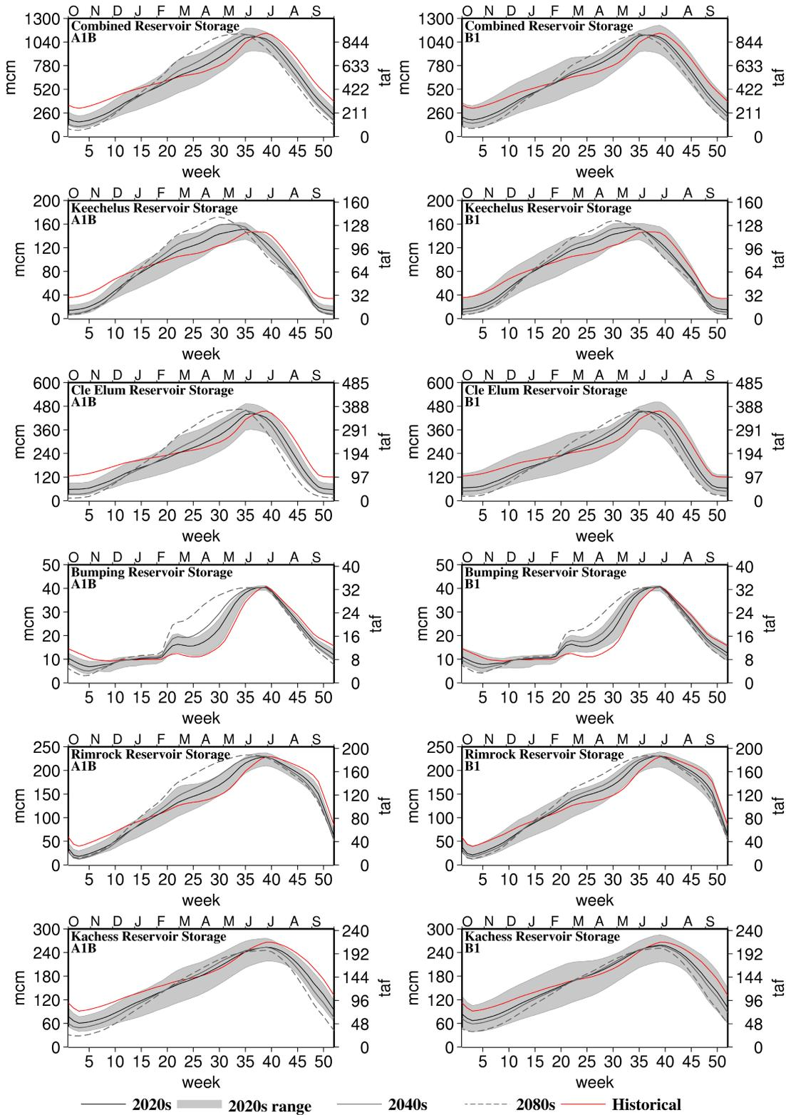
**Figure 7.** Reservoir storage. Simulated reservoir storage for the combined system (top panel) and for each of the five major reservoirs (lower five panels) for historical, 2020s, 2040s, and 2080s conditions.
