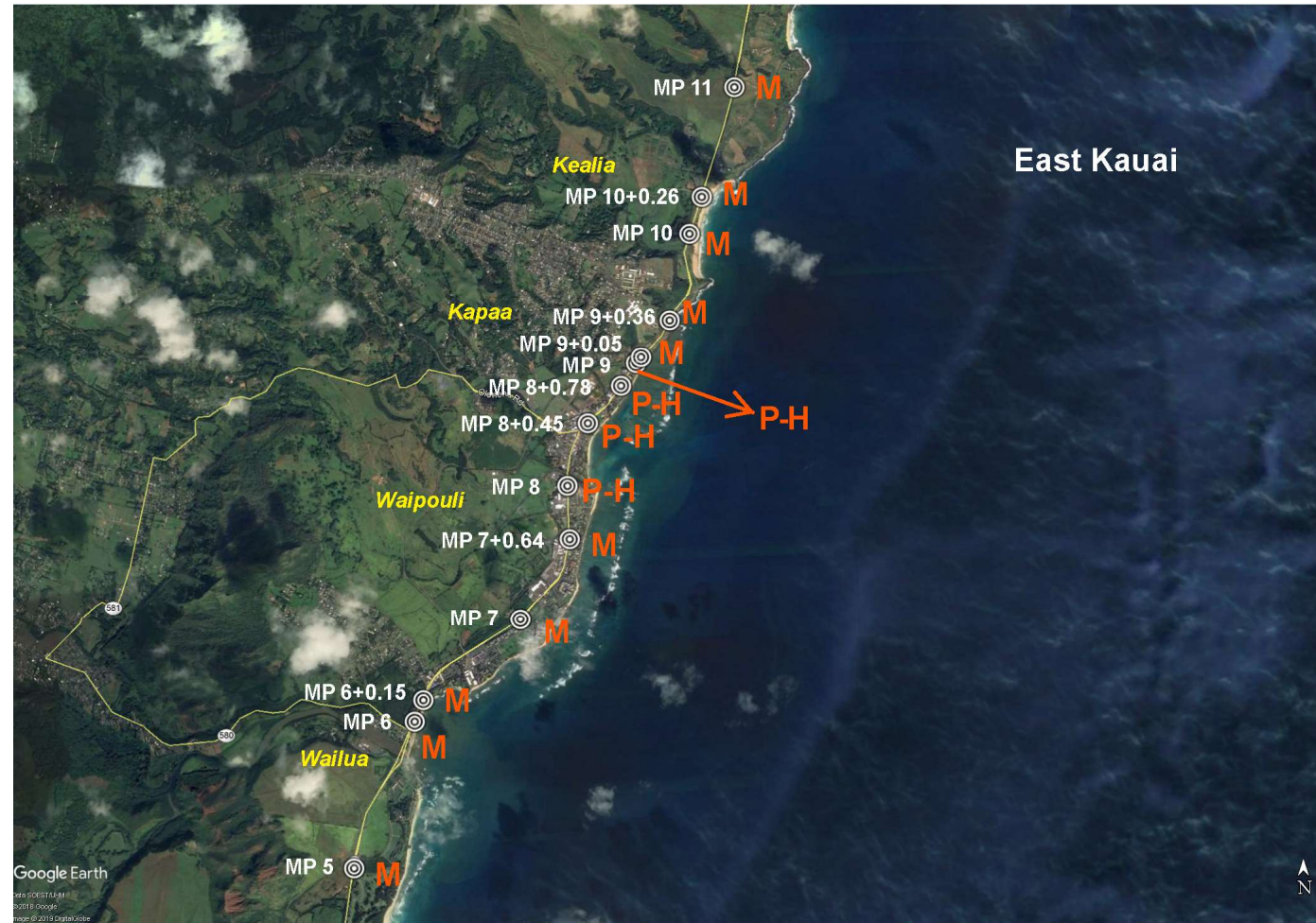
Figure 4.21. Wailua to Kealia adaptation recommendations for the State of Hawaii Statewide Coastal Highway Program Report (for table version, see Table 4.2). R-N is road relocation to new road; P-SD is living dunes; P-H is hard protection; C-H-E is elevate/hard protection; C-H-SD is hard/soft protection; M is no action/monitor.
