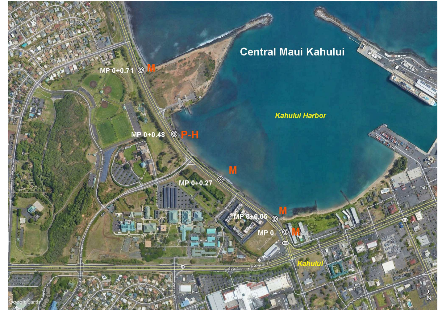
Figure 4.14. Kahului Harbor adaptation recommendations for the State of Hawaii Statewide Coastal Highway Program Report (for table version, see Table 4.2). R-N is road relocation to new road; P-SD is living dunes; P-H is hard protection; C-H-E is elevate/hard protection; C-H-SD is hard/soft protection; M is no action/monitor.
