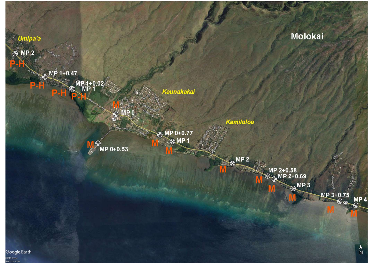
Figure 4.16. Kaunakakai area adaptation recommendations for the State of Hawaii Statewide Coastal Highway Program Report (for table version, see Table 4.2). R-N is road relocation to new road; P-SD is living dunes; P-H is hard protection; C-H-E is elevate/hard protection; C-H-SD is hard/soft protection; M is no action/monitor.
