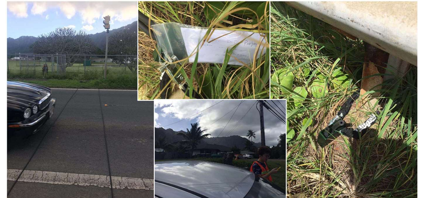
Figure 2.1. Typical traffic data collection using pneumatic road tubes collection, Oahu East Shore
