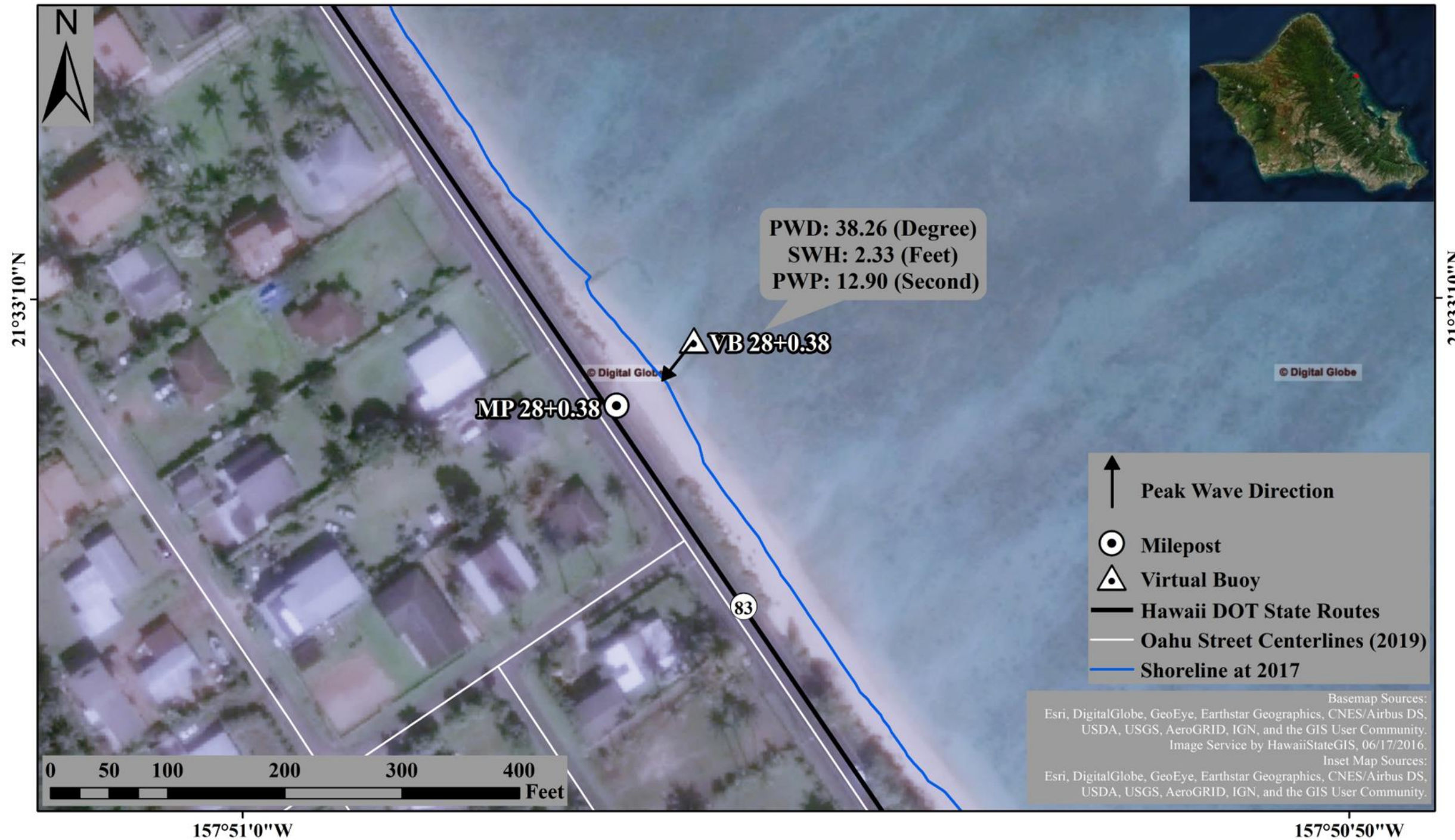
Figure 3.7. Sample map of maximum annually recurring wave information at Virtual Buoy (VB) 28+0.38, SR 83, East Shore, Oahu (Francis et al., 2019). Map of maximum annually recurring wave information at Virtual Buoy (VB) 28+0.38, SR 83, perpendicular to the State of Hawaii Department of Transportation (HDOT) route 83 at Milepost (MP) 28+0.38, SR 83, East Shore, Oahu. PWD represents Peak Wave Direction, from which the wave is coming, SWH represents Significant Wave Height, and PWP represents Peak Wave Period. Virtual Buoys (VB) are identified by Francis et al. (2019), and Mileposts (MP) are identified by Brandes et al. (2019). HDOT state routes and Oahu street centerline datasets are acquired from HDOT (2017) and HOLIS, C&CH (2017). Shoreline datasets are provided by NGS (2017). The maximum annually recurring wave information is available at Francis et al. (2019), which is derived according to the method presented in Anderson et al. (2018) and Vitousek & Fletcher (2008).
