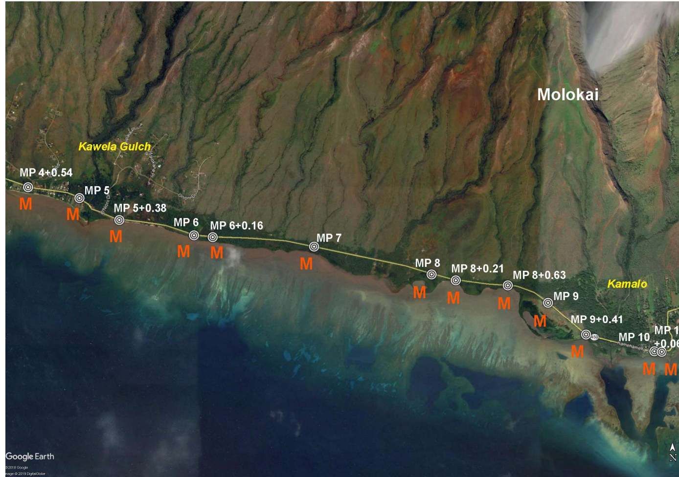
Figure 4.17. Kawela Gulch to Kamalo adaptation recommendations for the State of Hawaii Statewide Coastal Highway Program Report (for table version, see Table 4.2). R-N is road relocation to new road; P-SD is living dunes; P-H is hard protection; C-H-E is elevate/hard protection; C-H-SD is hard/soft protection; M is no action/monitor.
