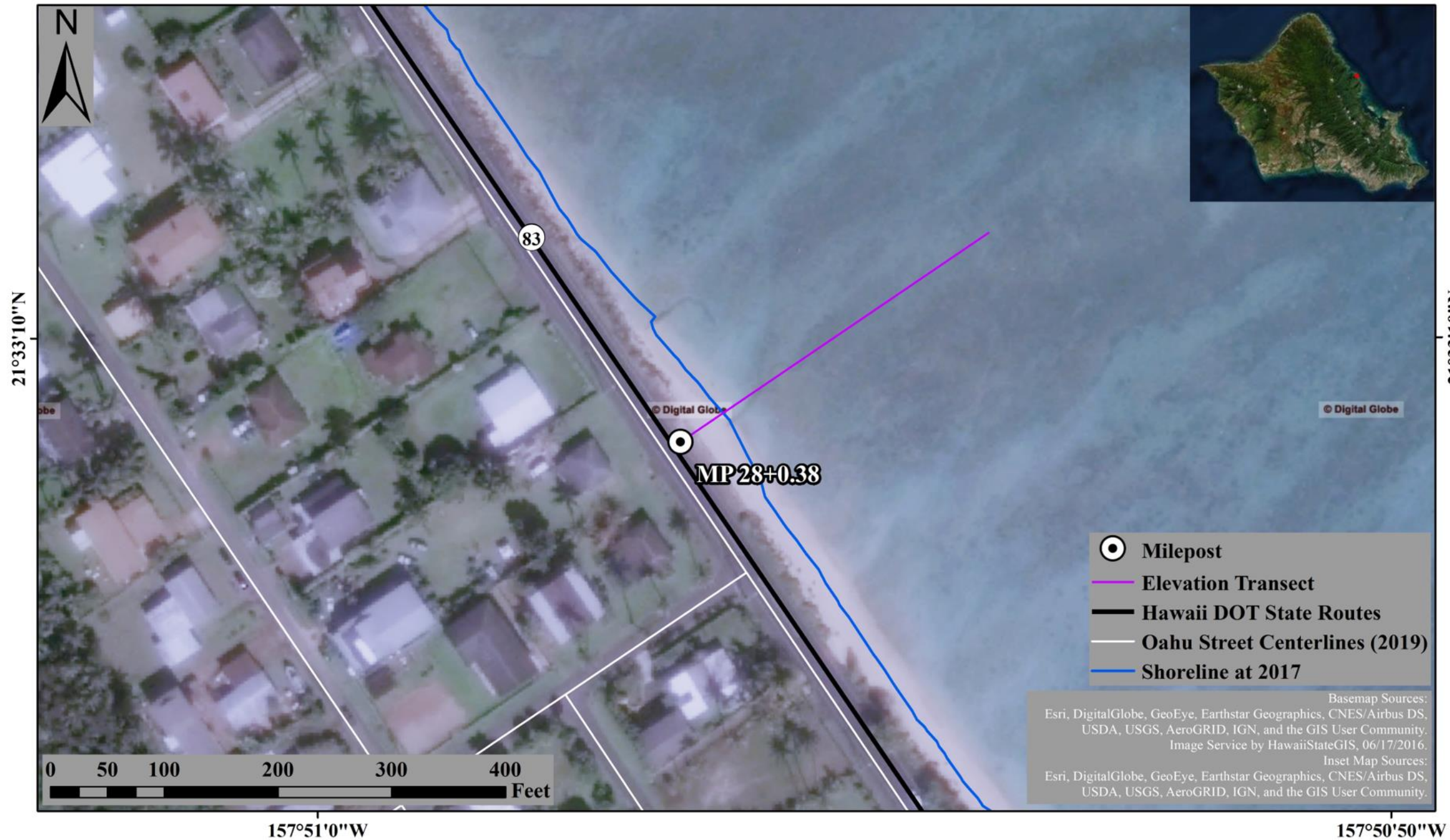
Figure 3.2. Sample map and plot of combined topographic and nearshore bathymetric transect at MP 28+0.38, SR 83, East Shore, Oahu (Francis et al., 2019). (a) Map and (b) plot of combined topographic and nearshore bathymetric transect perpendicular to the State of Hawaii Department of Transportation (HDOT) route 83 at Milepost (MP) 28+0.38, SR 83, East Shore, Oahu. Mileposts are identified by Brandes et al. (2019). HDOT state routes and Oahu street centerline datasets are acquired from HDOT (2017) and HOLIS, C&CH (2017). Elevations along the transect are referenced to local mean sea level (LMSL) and are sampled from a merged digital elevation model (DEM) of Oahu prepared by Francis et al. (2019).
