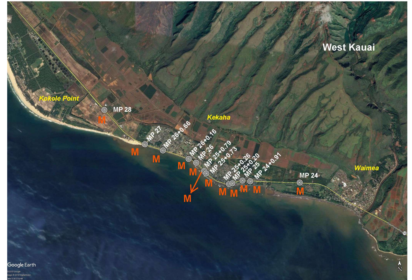
Figure 4.20. Waimea to Kokole Point adaptation recommendations for the State of Hawaii Statewide Coastal Highway Program Report (for table version, see Table 4.2). R-N is road relocation to new road; P-SD is living dunes; P-H is hard protection; C-H-E is elevate/hard protection; C-H-SD is hard/soft protection; M is no action/monitor.
