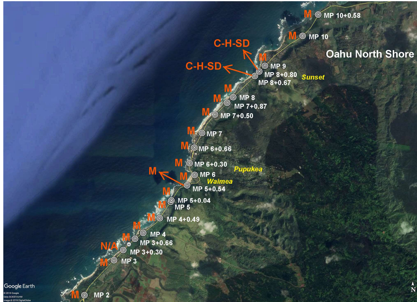
Figure 4.9. Oahu North Shore adaptation recommendations for the State of Hawaii Statewide Coastal Highway Program Report (for table version, see Table 4.2). R-N is road relocation to new road; P-SD is living dunes; P-H is hard protection; C-H-E is elevate/hard protection; C-H-SD is hard/soft protection; M is no action/monitor.
