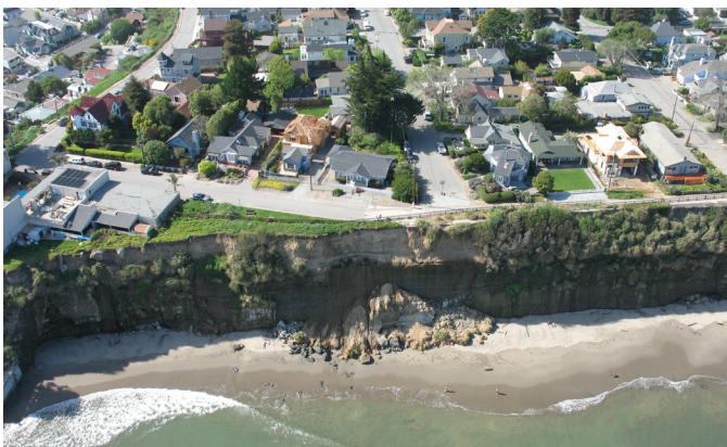
Figure 3.22. Cliff failure on Depot Hill, Capitola.
