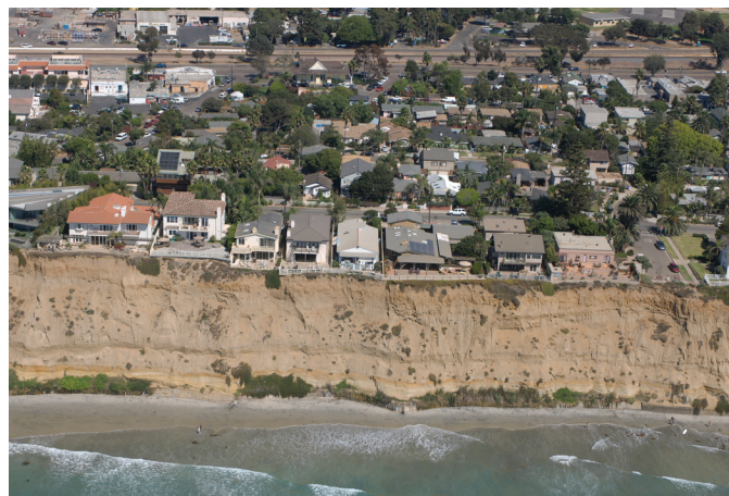
Figure 3.24. Lack of a fronting beach leads to continuous wave attack. A small rise in sea level will in all likelihood have a significant impact on cliff erosion in such areas (Kenneth and Gabrielle Adelman, California Coastal Records Project).
