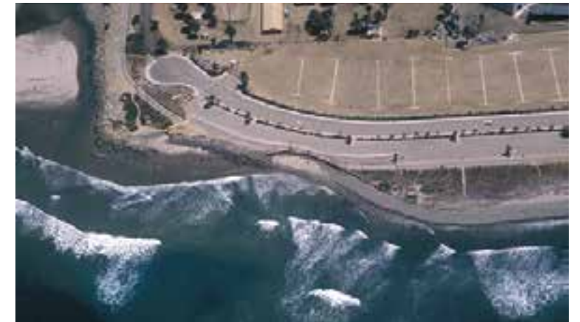
Before project construction: Coastal erosion had destroyed a bike path and damaged a parking area for the Ventura County Fairgrounds.
