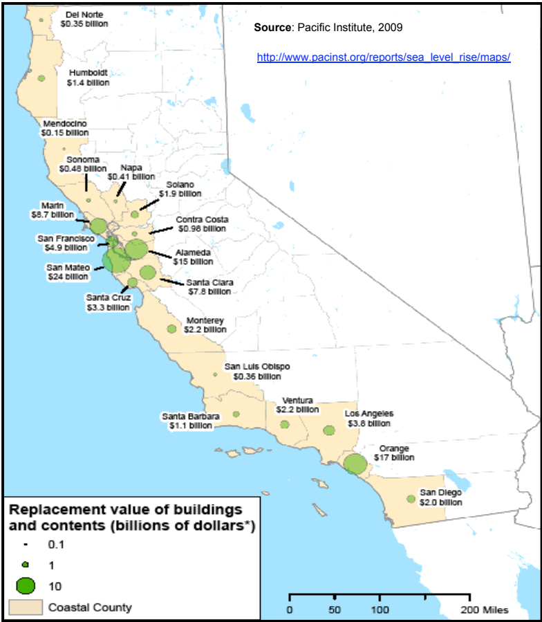
Figure 2: Replacement value of buildings and contents vulnerable to a 100 year coastal flood with 1.4 meters of sea level rise. Land values and relocation costs due to coastal erosion are not included.
