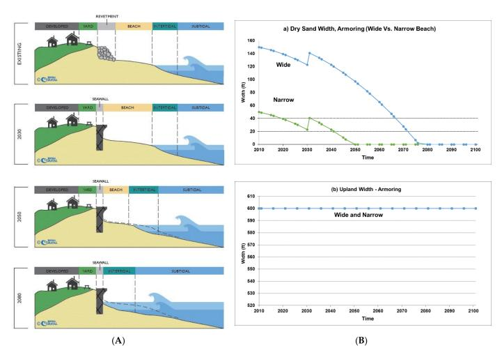
**Figure 8.** (**A**) Evolution of the armoring adaptation strategy, showing a small increase in usable beach as the existing revetments are replaced with vertical seawalls, then the loss of dry and eventually intertidal sand beaches over time. (**B**) Dry sand beach width over time with armoring (wide vs. narrow beach) (Ba top plot); upland width over time with armoring (wide vs. narrow beach) (Bb bottom plot).
