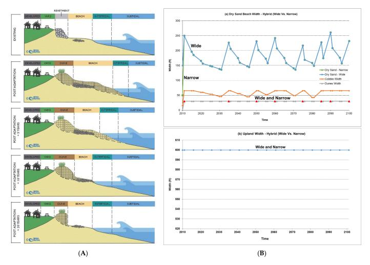
**Figure 10.** (**A**) Evolution of the living cobble and dune shoreline strategy over time. Example does not illustrate the shortening time between nourishment cycles as sea level rises. (**B**) Dry sand beach width over time with armoring (wide vs. narrow beach) (Ba top plot); upland width over time with armoring (wide vs. narrow beach) (Bb bottom plot).
