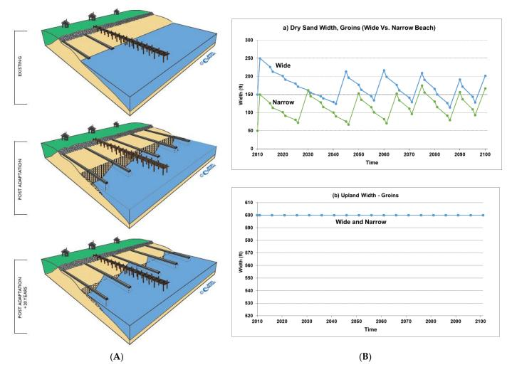
**Figure 11.** (**A**) Sand retention with groins adaptation strategy over time. (**B**) Dry sand beach width over time with armoring (wide vs. narrow beach) (Ba top plot); upland width over time with armoring (wide vs. narrow beach) (Bb bottom plot).
