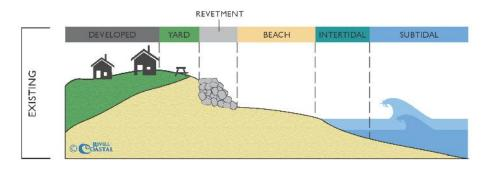
**Figure 5.** Conceptual model of physical upland and beach widths tracked as a result of adaptation strategy implementation over time. For this case study, developed and yard were considered as upland. The revetment in this figure was the adaptation project, while the beach, and intertidal were considered as the beach width.
