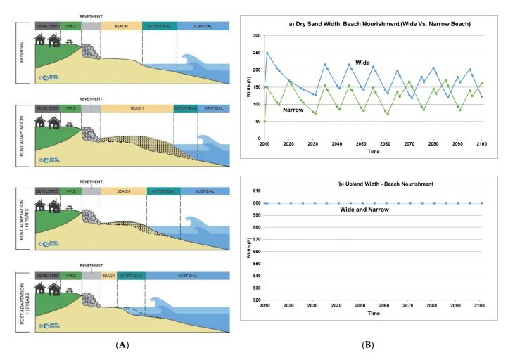
**Figure 9.** (**A**) Evolution of the beach nourishment strategy over time. Example does not illustrate the shortening time between nourishment cycles as sea level rises. (**B**) Dry sand beach width over time with armoring (wide vs. narrow beach) (Ba top plot); upland width over time with armoring (wide vs. narrow beach) (Bb bottom plot).
