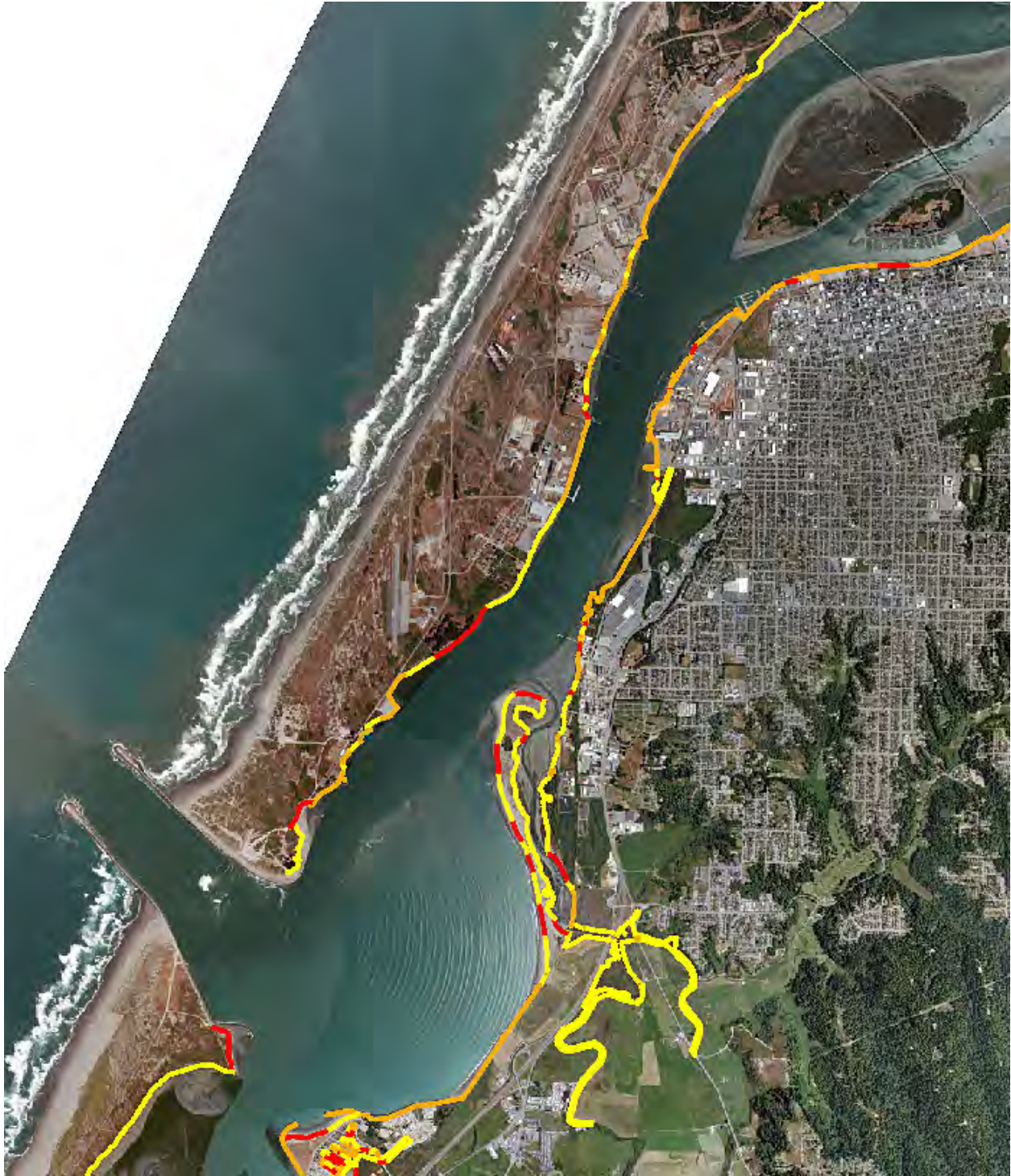
Figure 76. Eureka Bay shoreline cover: fortified (brown), vegetated (yellow), and exposed (red).
