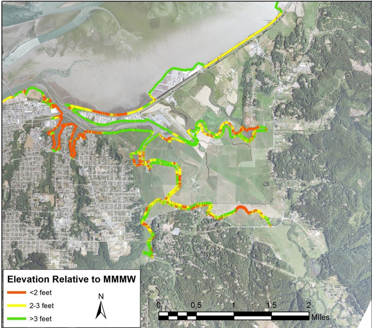
Figure 8. . Shoreline elevation above the MMMW elevation of 7.7 ft (NAVD 88): red <2 ft, yellow = 2-3 ft, and green > 3 ft, on Eureka Slough and Arcata Bay (Laird 2013).
