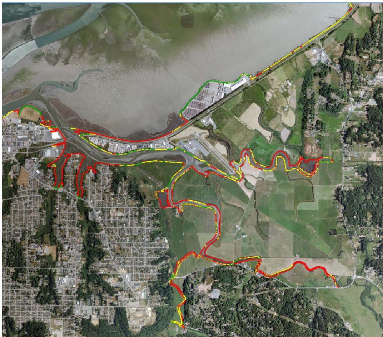
Figure 9. Shoreline vulnerability rating to erosion or overtopping on Eureka Slough: red is highly vulnerable, yellow-moderately, and green low.
