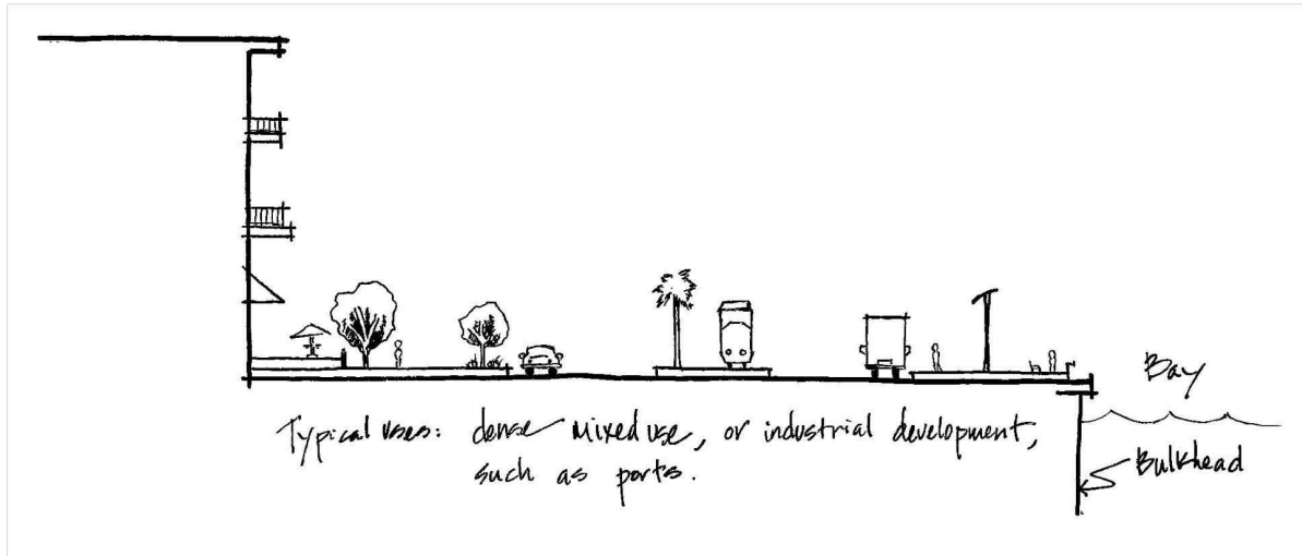
Figure 1.21 Typical Section: Urban Shoreline with Bulkhead
