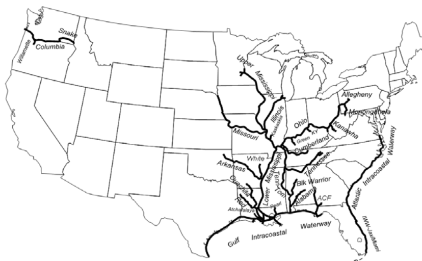
FIGURE 3-1 U.S. Fuel-Taxed Inland Waterway System. SOURCE: U.S. Army Corps of Engineers.
