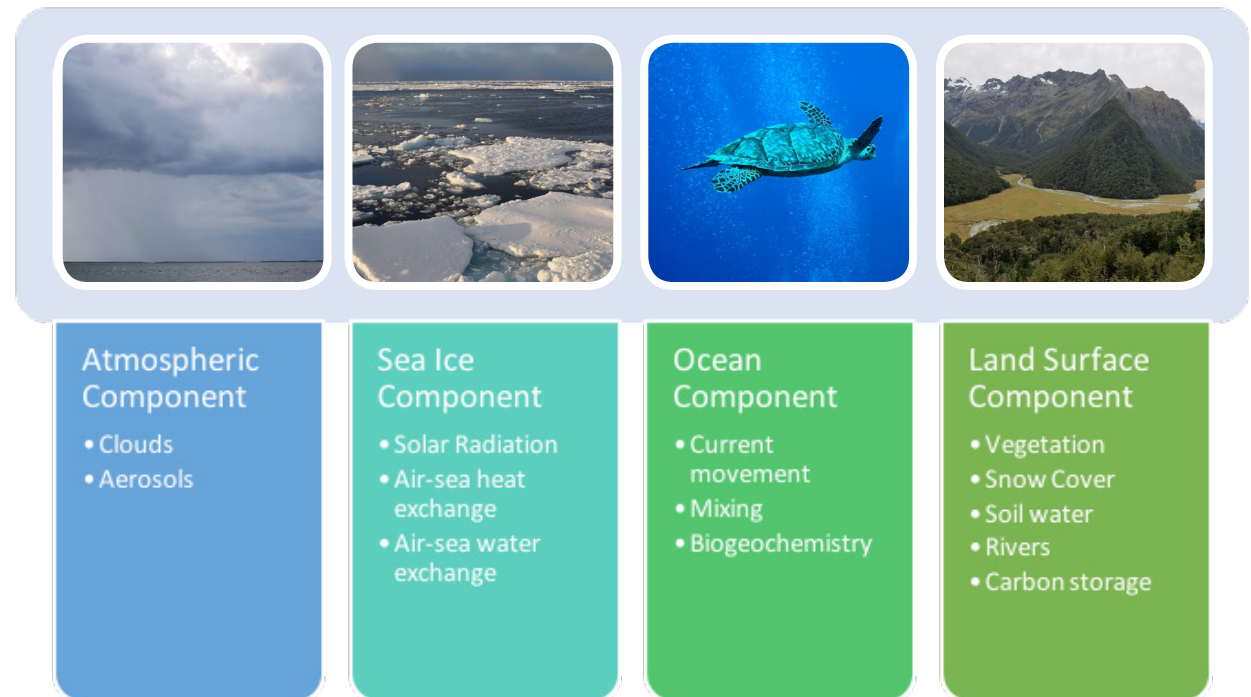
Figure 28. A Global Climate Model (GCM) is a complex mathematical representation of the major climate system components and their interactions. Earth's energy balance between the four components is the key to long-term climate prediction. Text from the Geophysical Fluid Dynamics Laboratory available at https://www.gfdl.noaa.gov/climate-modeling/
