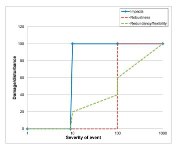
**Figure 3.** Severity-disruption relationship for a reference system and a system with added robustness, redundancy, and flexibility.
