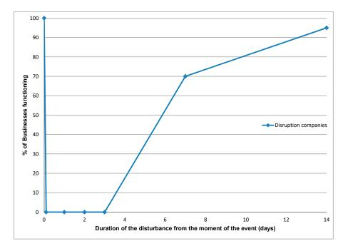
**Figure 7.** Disruption over time for the storyline scenario. The total disruption can be assessed by calculating the area between the 100% level and the blue curve. The total disruption is 34% of the total businesses functioning
