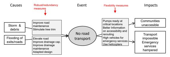
**Figure 9.** Road transport: causes, impacts, and potential measures which prevent disruption of road transport (in the grey blocks on the left side) or mitigate impacts (grey blocks on the right side).
