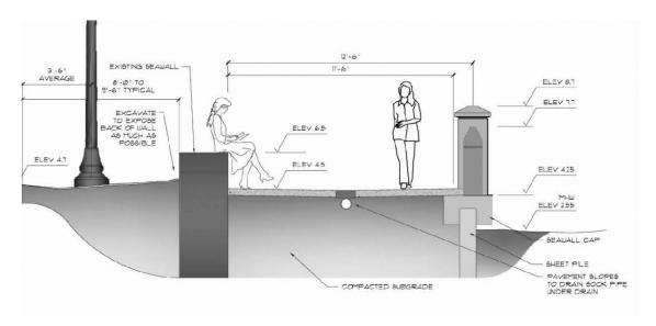
Fig. 42: The section of the current St. Augustine Seawall project illustrates the historic seawall on the left with the new, higher seawall on the right. Approximately two feet (61 centimeters) of the coquina seawall will be visible. This illustration does not depict the six-inch (15-centimeters) height increase for the new seawall and pedestrian path applied after severe flooding in November 2012. [City of St. Augustine; St. Augustine Seawall Flood Mitigation Project, August 22, 2011]
