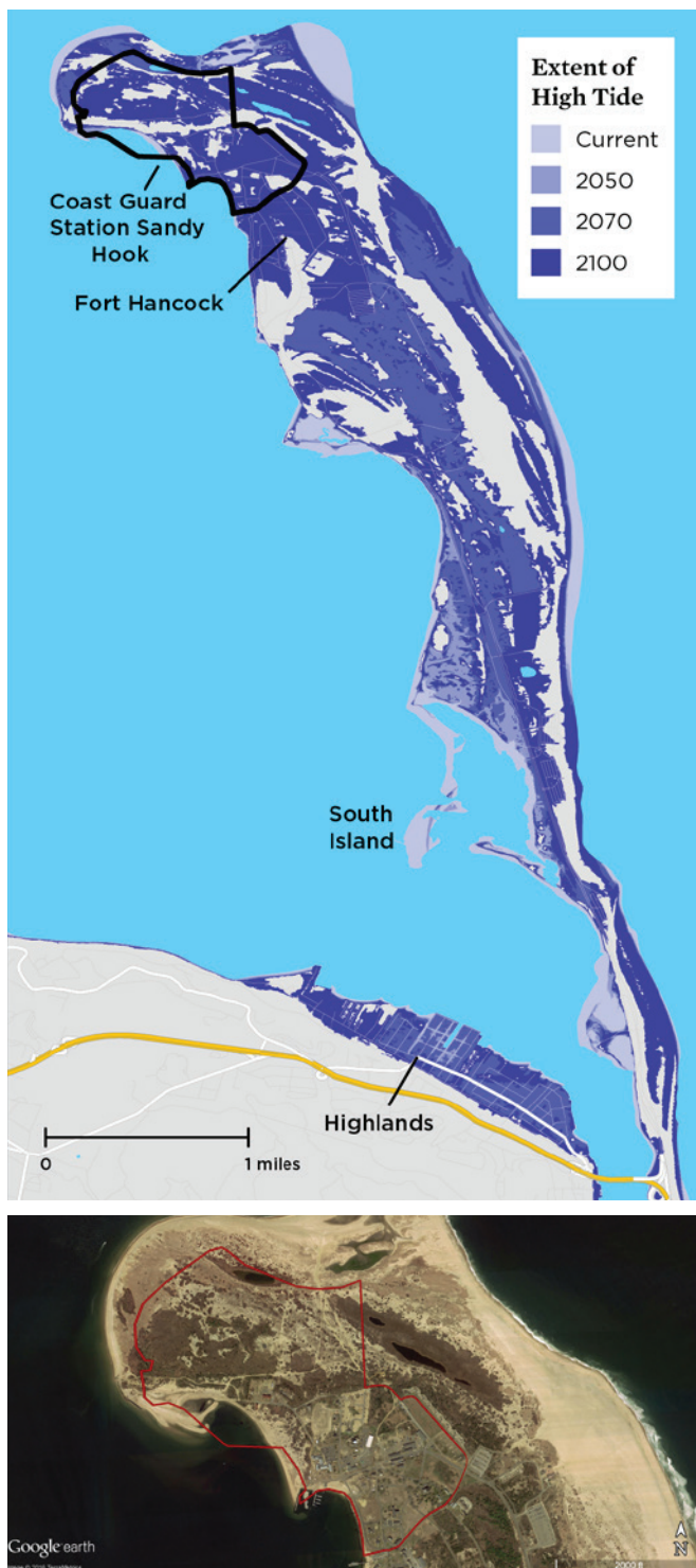
The projected reach of future daily high tides, shown above, encompasses currently utilized land at USCG Station Sandy Hook, shown on the bottom. The highest scenario is mapped here.
