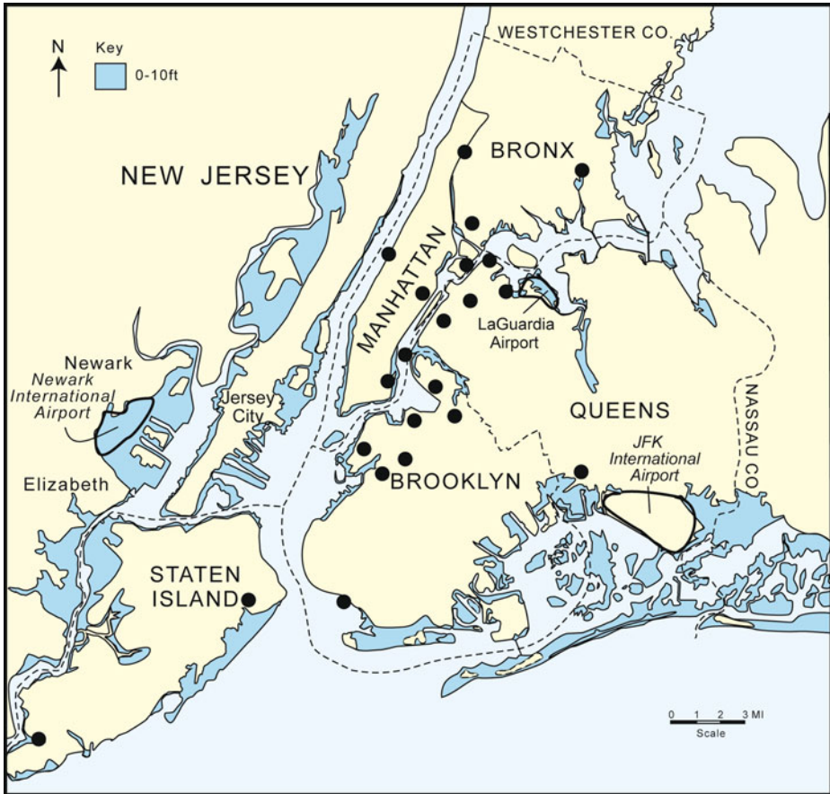
Fig. 7 Locations of New York City power plants relative to 10-ft elevation contour. Source: NPCC (2010)
