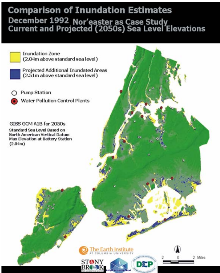
Fig. 5 Comparison of Nor'easter of 1992 and a sea level rise estimate of 47.2 cm for 2050
