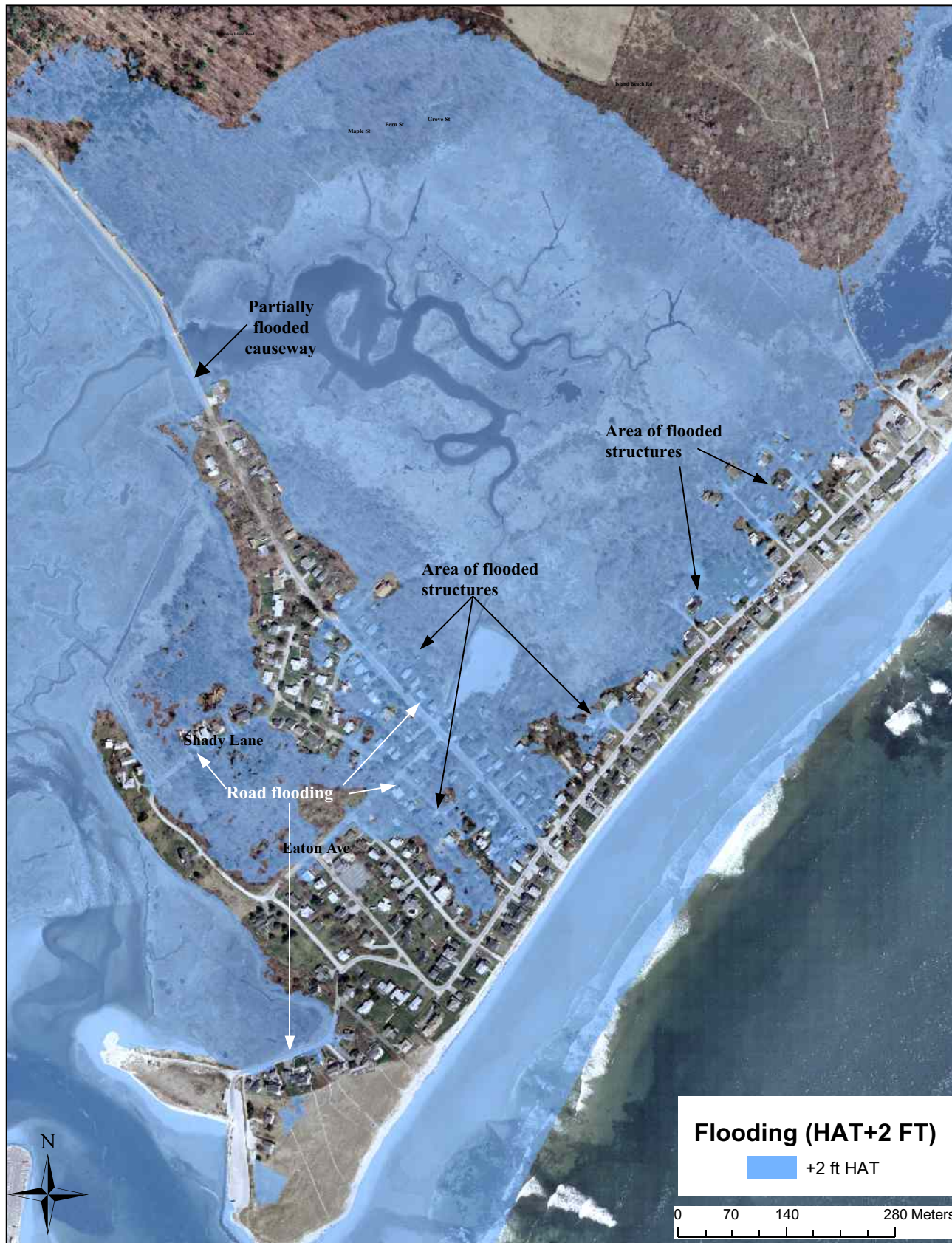
Figure 13. Simulated flooding of Drakes Island with 2 ft sea level rise at HAT conditions. Note that the causeway (Drakes Island Road) is now flooded. More extensive flooding occurs along the central portion of Drakes Island Road, Shady Lane, Eaton Avenue, and down Grove St. Isolated lots along Island Beach Road also undergo flooding.
