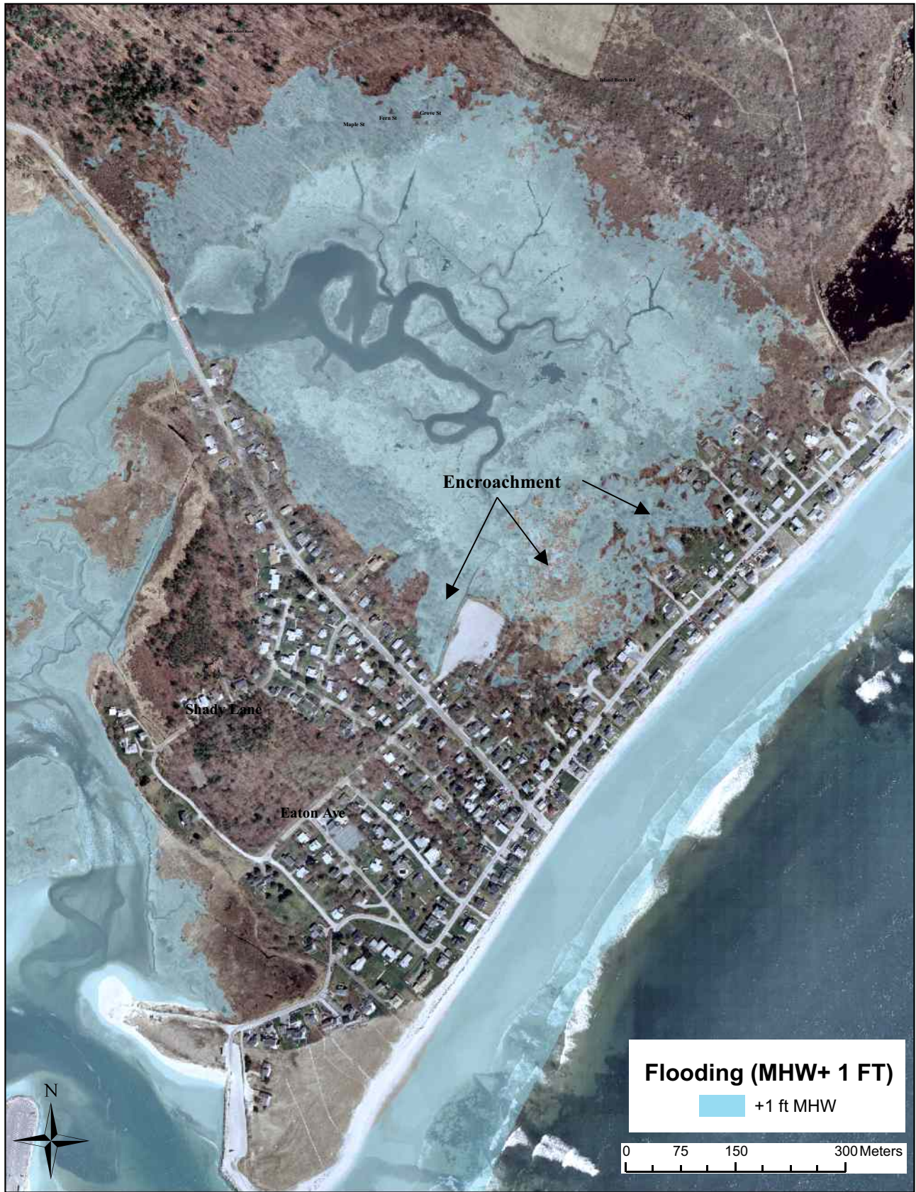
Figure 10. Simulated flooding of Drakes Island after 1 ft of sea level rise under MHW conditions. Note the encroachment of flood waters near private property (and a public parking lot) northeast of Drakes Island Road and northwest of Island Beach Road.
