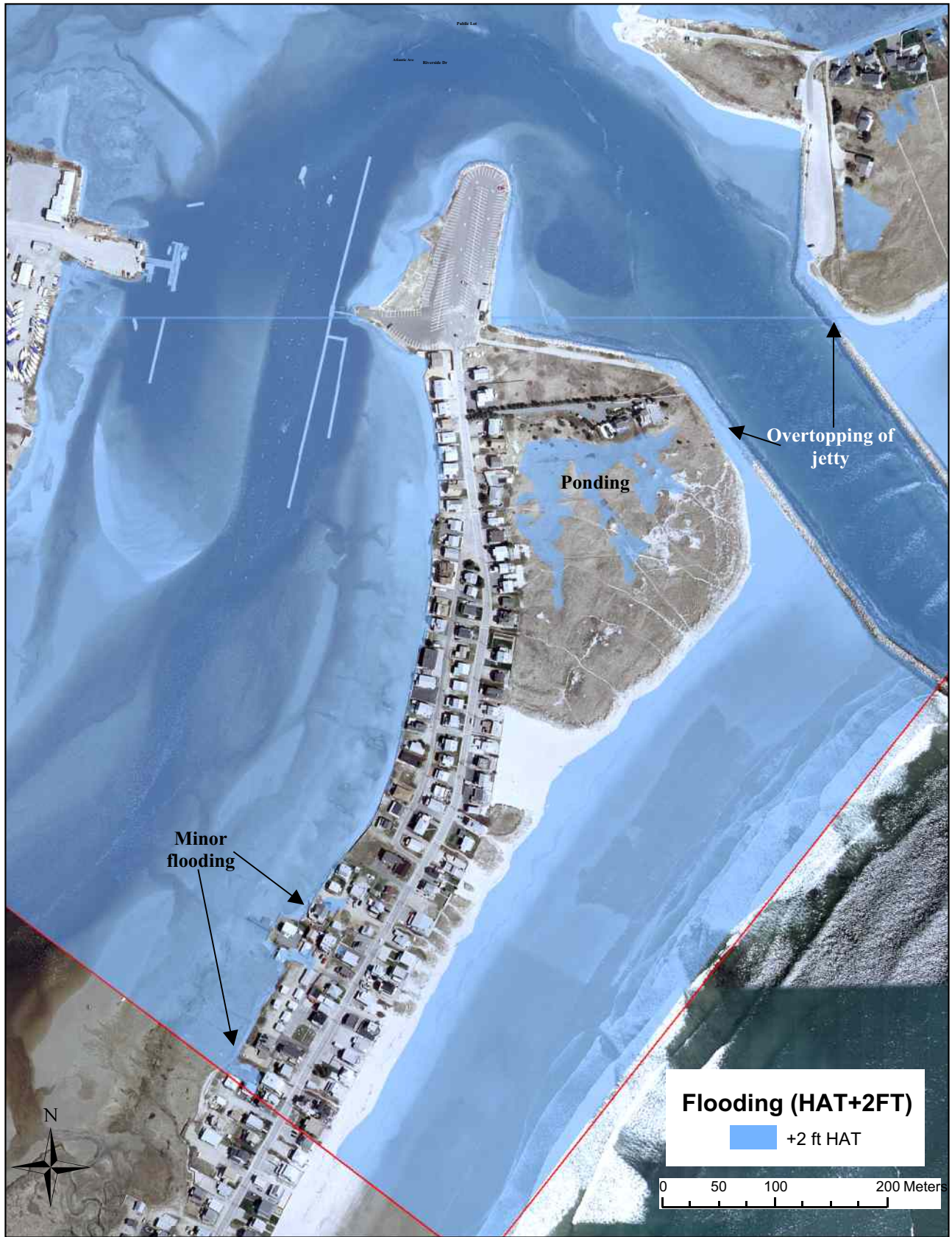
Figure 14. Simulated flooding for Wells Beach with 2 ft rise in sea level at HAT conditions. Only minor flooding is apparent on the marsh (Webhannet River) side of the island, where several low-lying areas are flooded. Portions of the existing jetties are also overtopped.
