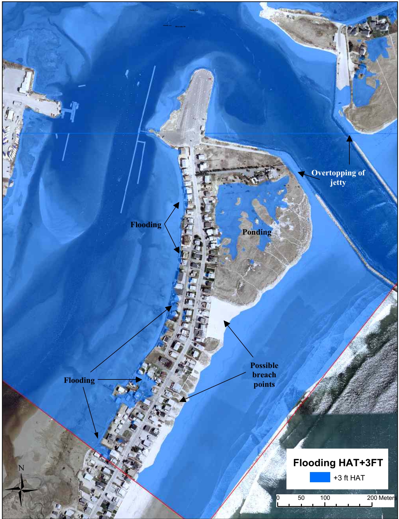
Figure 17. Simulated flooding of Wells Beach for 3ft sea level rise at HAT conditions. More extensive overtopping of the seawalls would occur, resulting in more flooding along the Webhannet River side of the island. More extensive ponding adjacent to the jetties occurs, and several breach points become more apparent.
