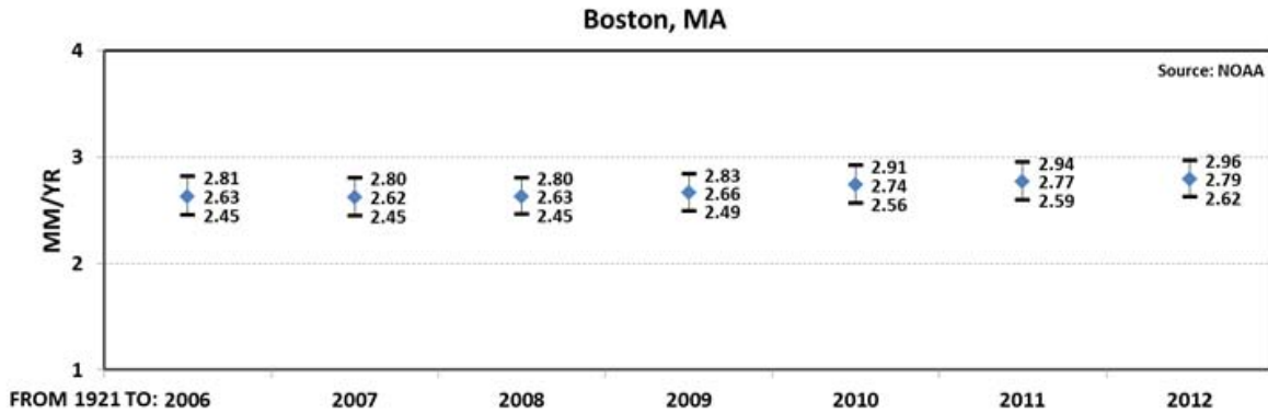
Figure 2. Mean sea level rates (blue diamonds) and 95% confidence intervals (in millimeters per year) calculated from 1921 to recent years (2006-2012) at the NOAA Boston tide gauge station. Values are the trend of the entire data period up to that year.
