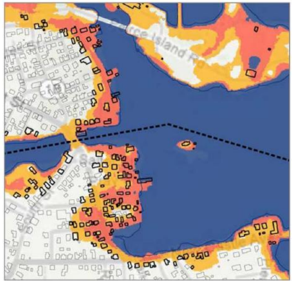
Stillwater Elevation 11.5 Feet NAVD
