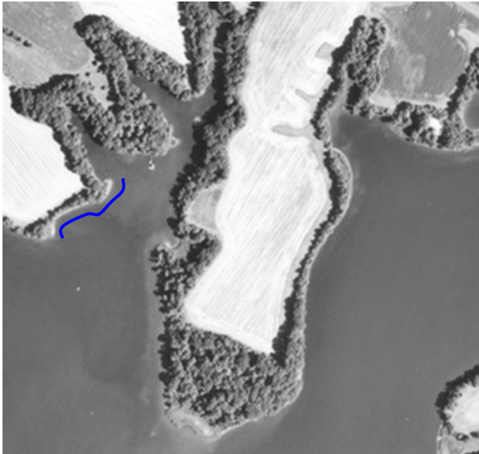
Figure 5. Aerial View of Wye NRMA site. The groins at Wye NRMA do not seem to extend far enough into the water to trap the sediment being transported by longshore currents. As a result, a sand spit is forming at the eastern end of the project (arrow). Perhaps only fetch and wave climate were considered when designing this structure but boat-generated waves appear to also be quite significant at this site.
