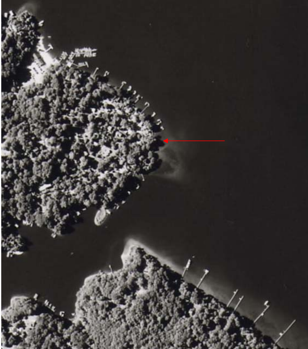
Figure 8. Aerial view of the Epping Forest Site. Note the sediment fan just south of the vegetated breakwater (red arrow).
