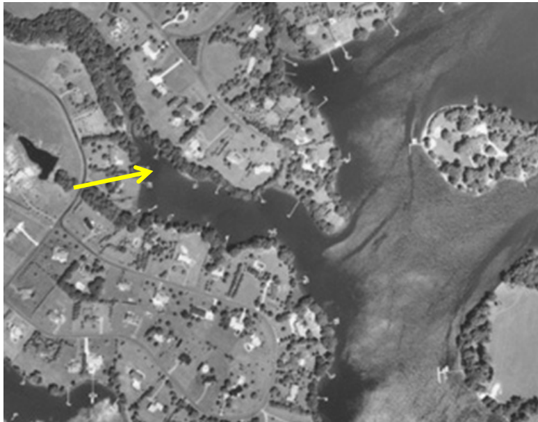
Figure 3. Aerial view of Elliott R. Site. The groins at Elliott R.'s were located in a relatively quiescent creek with very soft sediments. Long shore transport appears to be minimal leading to no or little trapping of sediment by the structures. Instead, the sand deposited in the marsh zone may be lost once resuspended (see text).
