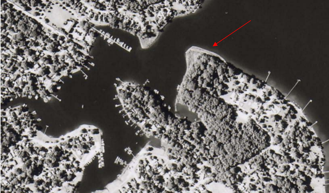
Figure 10. Aerial view of the London Town Site. Note the lack of sediment patterns adjacent to the structure but their presence SE of the breakwater.
