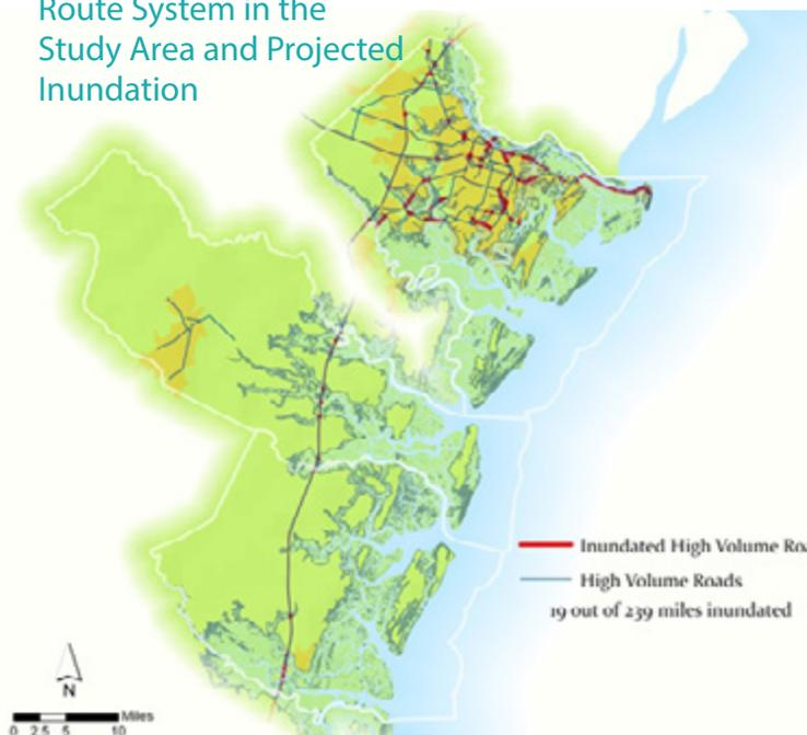
Figure 2.32- Existing High Volume Roads in Study Region and Projected Inundation
