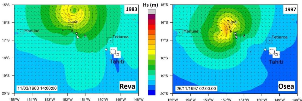
Figure 6. Examples of wave modeling for two cyclones affecting the Society islands. Colors show significant wave heights during the event while arrows show waves' directions. This modeling shows Reva (left) affecting the eastern side of Tupai while Osea hit the western side. For each cyclone in the JTWC database, the complete sequence of cyclonic waves was computed.
