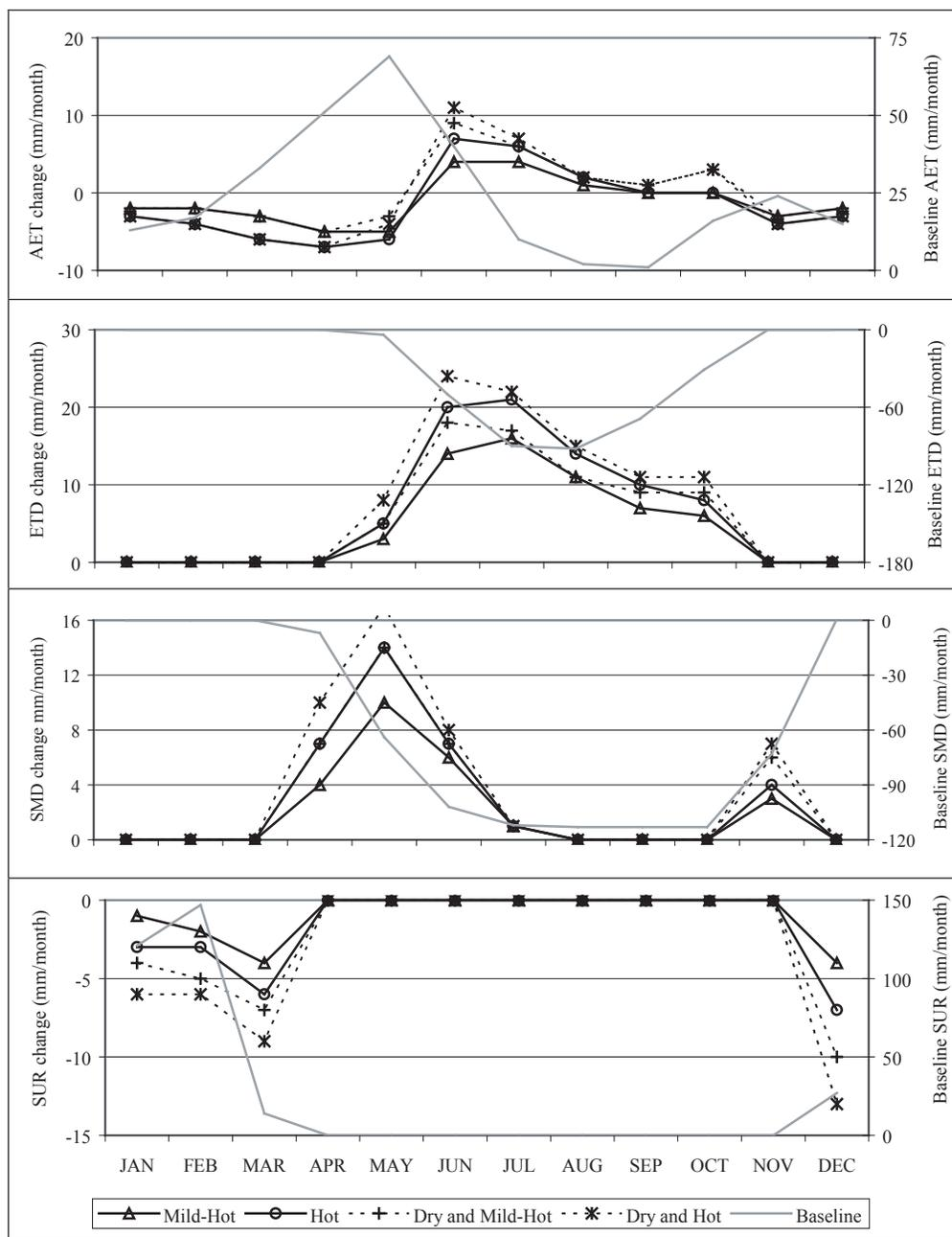
**Fig. 5.** Climate change impact on water balance parameters in Ksara, Lebanon. Baseline results are plotted as absolute values on the right-hand side vertical axis. Scenario results are plotted as changes from baseline values (scenario–baseline) on the left-hand side vertical axis. AET=actual evapotranspiration, ETD=evapotranspiration deficit, SMD=soil moisture deficit, and SUR=water surplus.
