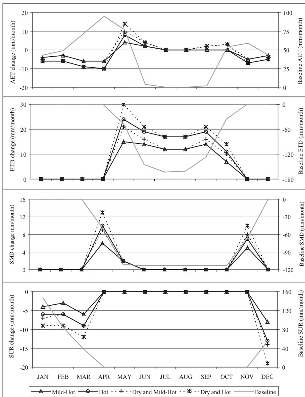
**Fig. 4.** Climate change impact on water balance parameters in Beirut, Lebanon. Baseline results are plotted as absolute values on the right-hand side vertical axis. Scenario results are plotted as changes from baseline values (scenario–baseline) on the left-hand side vertical axis. AET=actual evapotranspiration, ETD=evapotranspiration deficit, SMD=soil moisture deficit, and SUR=water surplus.
