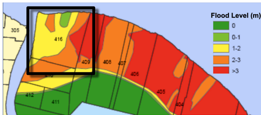
Fig. 3. Illustration of the disproportionate extent and depth (in meters) of flooding in Georgetown (represented by section 416—indicated by black box) in January 2005
