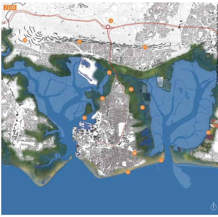
The M27 that served as the east to west link across the south coast – from Southampton to Chichester – was relocated to safer ground behind the hills to the north of the city. Although this relocation was costly, it was a smaller investment than protecting the existing route from long-term flooding.
