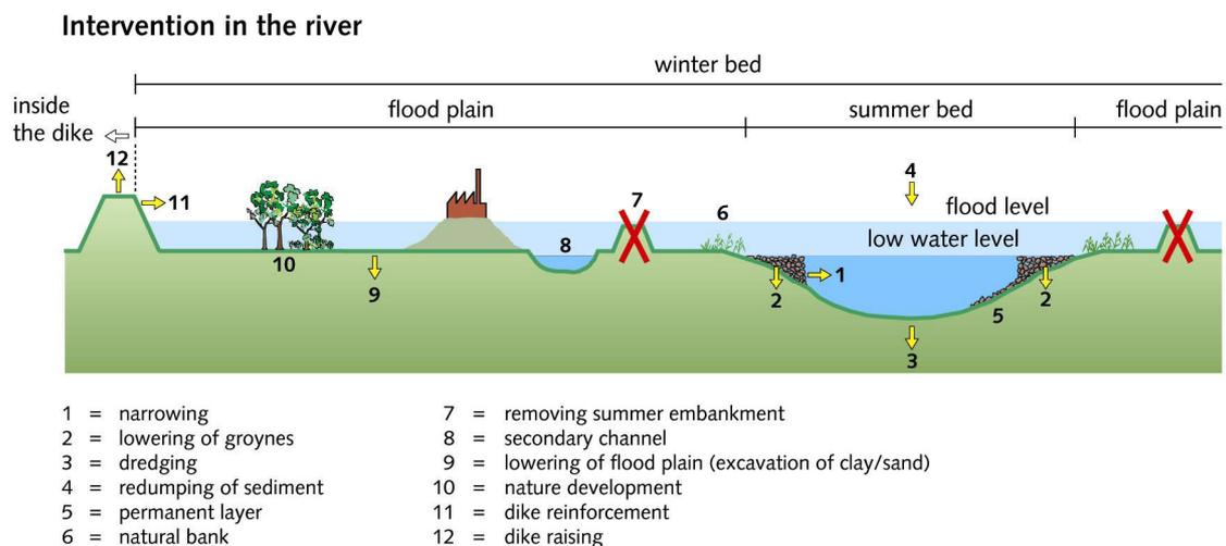
Figure 3-2 Schematic representation of measures being planned and executed in the programmes 'Room for the Rivers' and 'Maaswerken'
