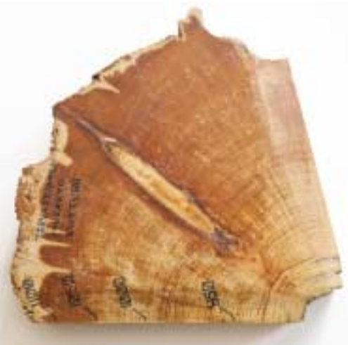
The climatic information of annual rings are preserved in tree trunks in the bottoms of cold lakes in Lapland for more than 7000 years. This section of a Scots pine stump was found in a forest stand in western Lapland, 800 years after the death of the tree.
