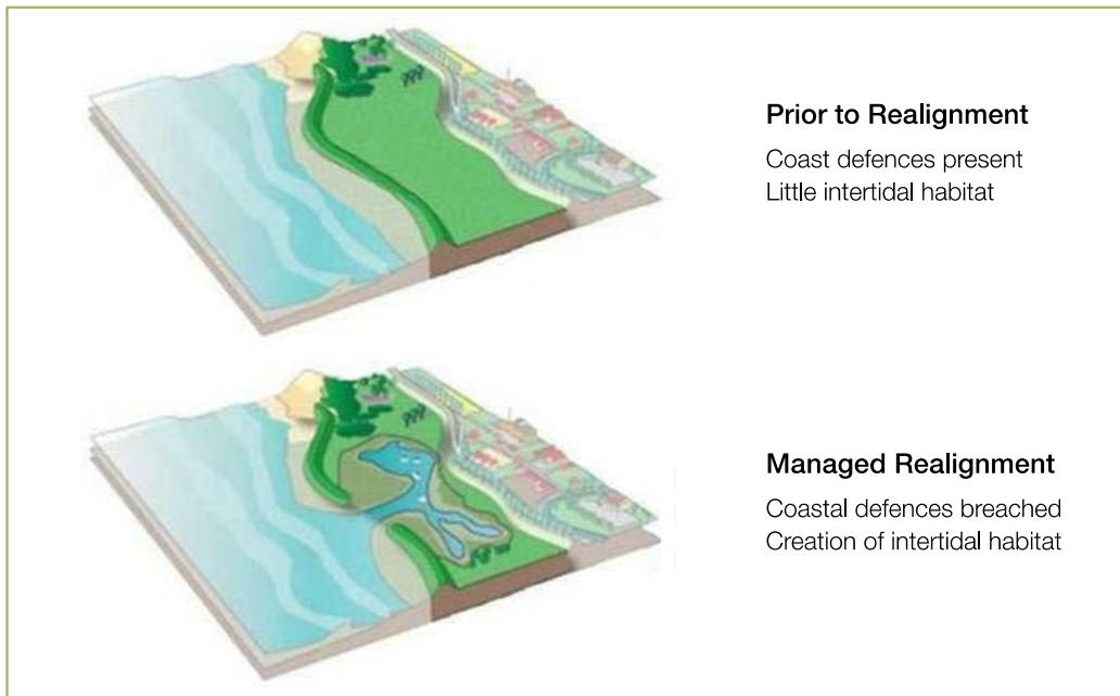
Figure 93: Mechanisms of managed realignment (Adapted from: Linham & Nicholls, 2010).
